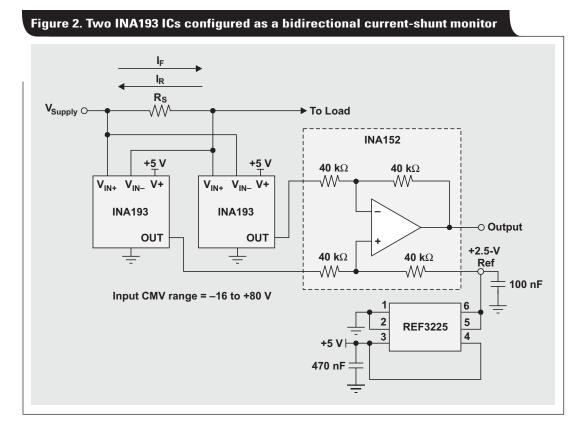
flow in the correct direction. Two of the unidirectional current-shunt-monitor ICs may be interconnected to form a bidirectional current-shunt monitor with a CMV range that extends from -16 to +80 V. The addition of the INA152 instrumentation amplifier and +2.5-V reference completes the circuit. A circuit schematic for the INA193 bidirectional current-shunt monitor is shown in Figure 2.
