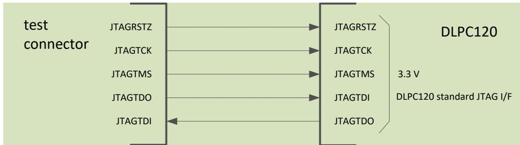
**Figure 8-3. DLPC120-Q1 JTAG Boundary Scan Connection Example**
