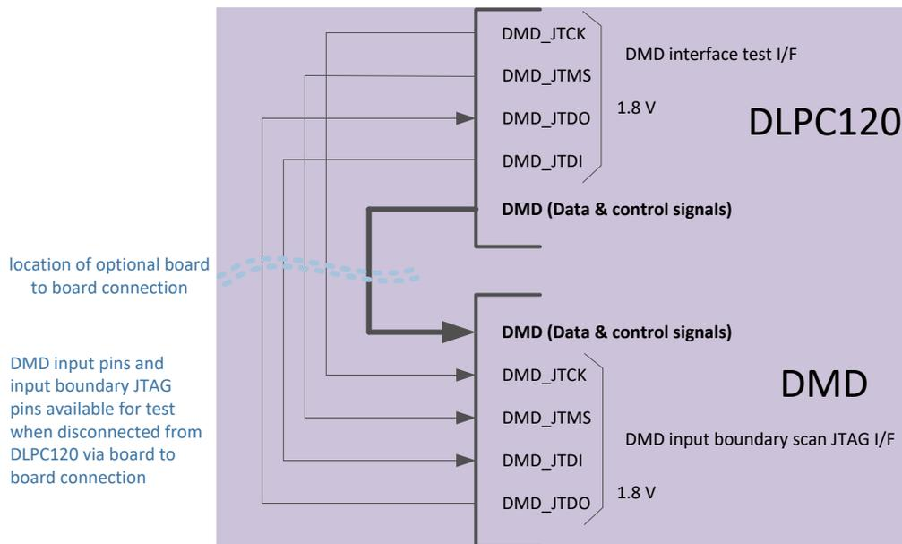
**Figure 8-4. DLPC120-Q1 JTAG to DMD Interface Connection Example**
