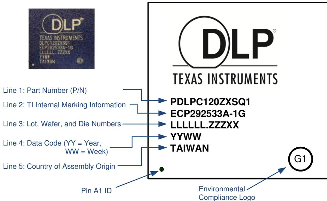
**Figure 12-1. Device Marking**
