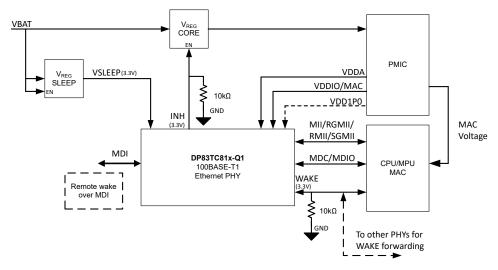
Figure 5-4. System Block Diagram
