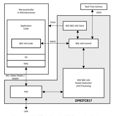
Figure 5-2. DP83TC817 Example PTP System Application
