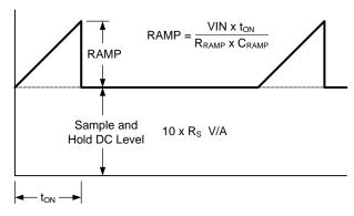
Figure 9. Composition of Current Sense Signal
