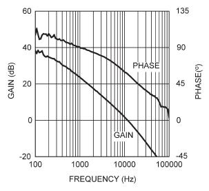
Figure 20. Overall Voltage Loop Gain and Phase
