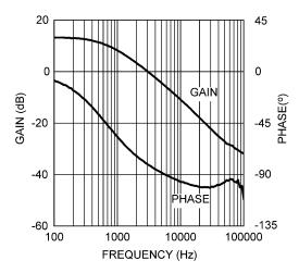
Figure 18. Modulator Gain and Phase
