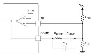
Figure 16. Feedback Configuration
