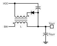
Figure 8. VCC Bias Supply With Additional Inductor Winding
