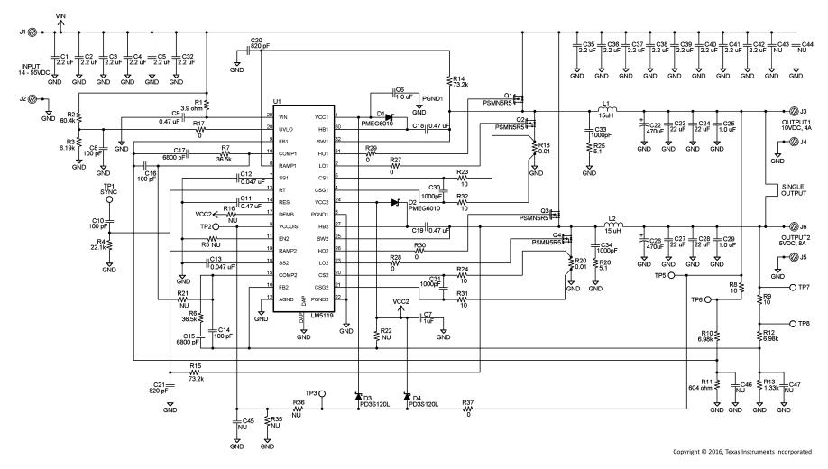
Figure 14. 10-V 4-A, 5-V 8-A Dual Output Application
