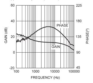
Figure 19. Error Amplifier Gain and Phase
