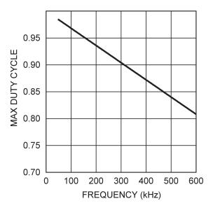
Figure 11. Maximum Duty Cycle vs Switching Frequency
