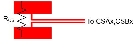
(a) Kelvin Connect of Resistor without Sense Pins
