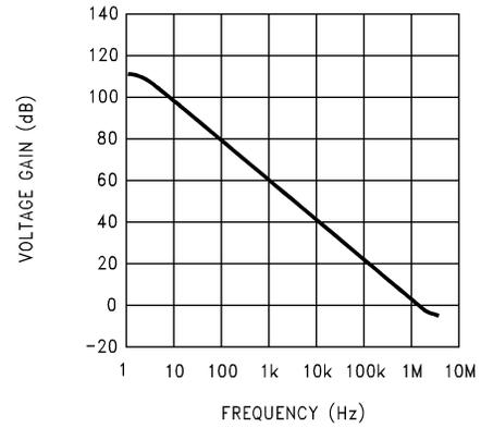
**Figure 5-10. Open-Loop Frequency Response**
