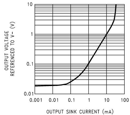
Figure 5-6. Output Characteristics Current Sinking
