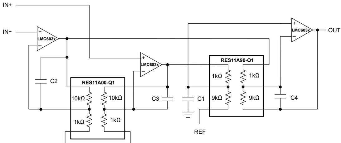
**Figure 6-7. Improved Instrumentation Amplifier With RES11A**
