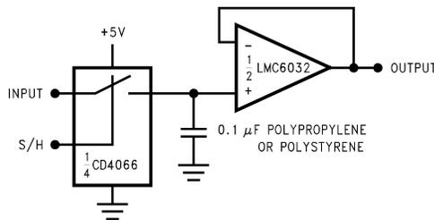
**Figure 6-9. Low-Leakage Sample-and-Hold**
