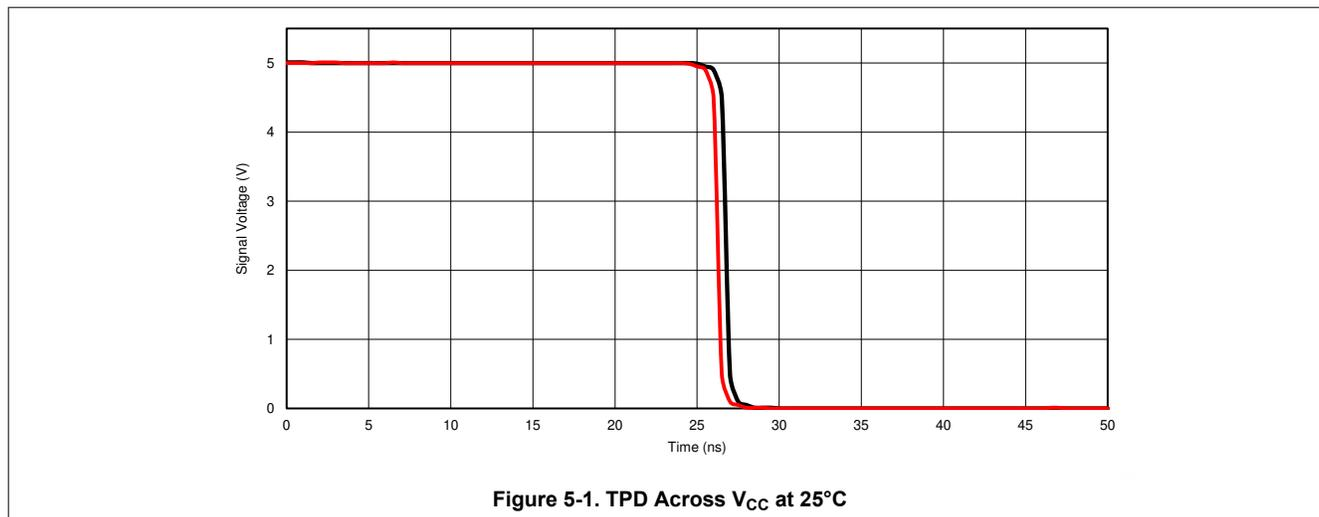
Figure 5-1. TPD Across  $V_{CC}$  at  $25^\circ\text{C}$
