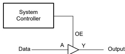
**Figure 9-1. Typical Application Block Diagram**
