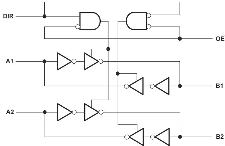
Logic Diagram (Positive Logic) for 1/2 of SN74AVC4T245-Q1
