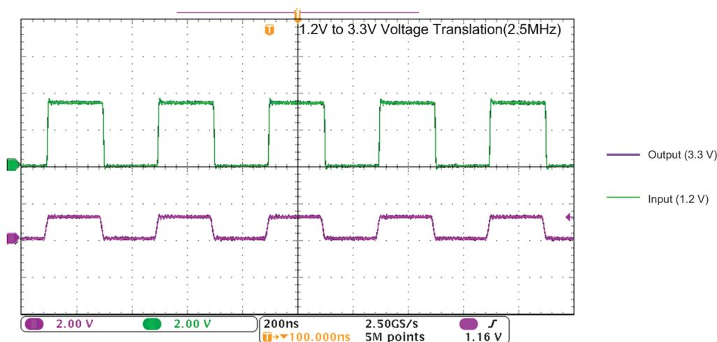
**Figure 8-2. Translation Up (1.2V to 3.3V) at 2.5MHz**
