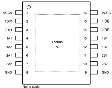
Figure 4-4. DYY Package, 16-Pin SOT (Top View)
