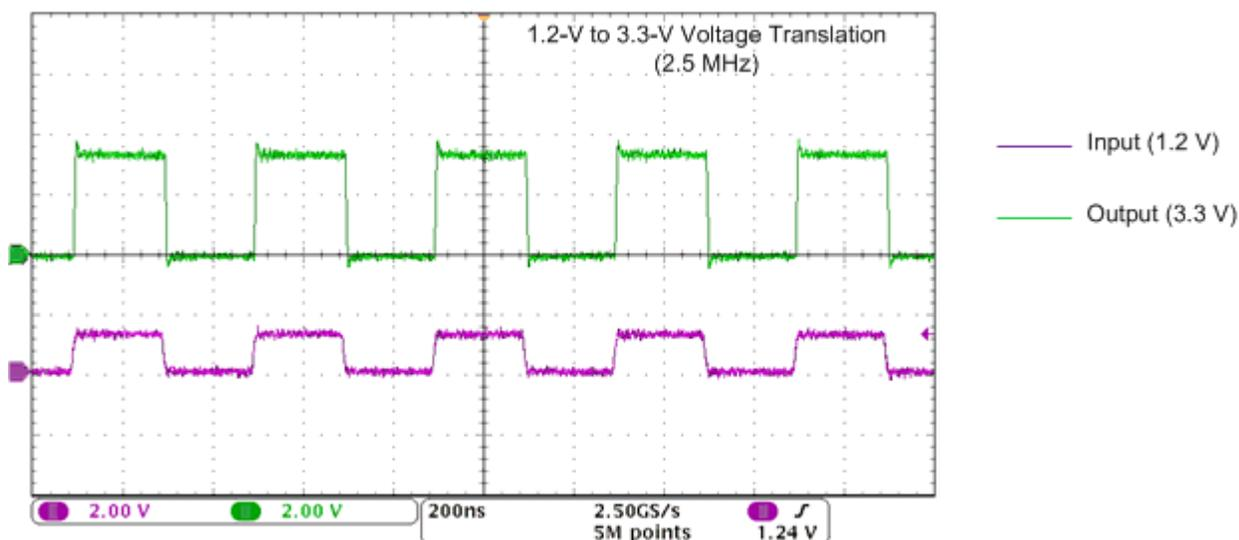
**Figure 9-2. Translation Up (1.2V to 3.3V) at 2.5MHz**
