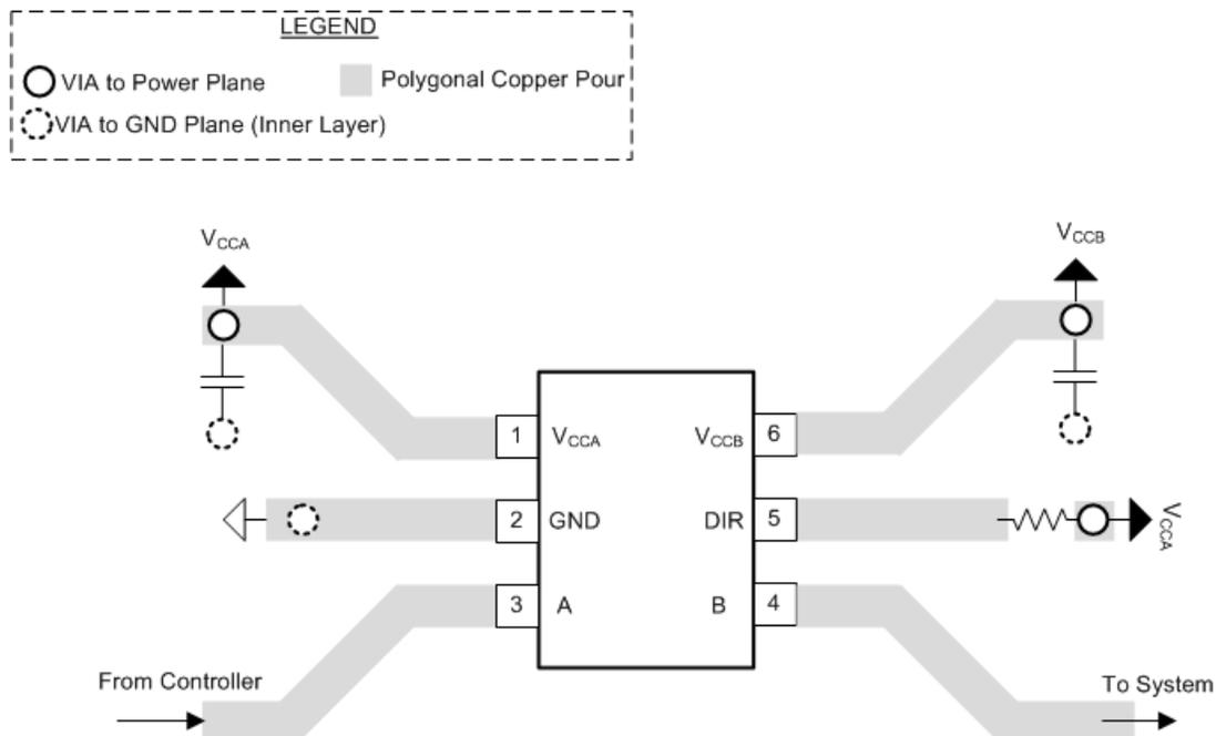
Figure 11-1. PCB Layout Example
