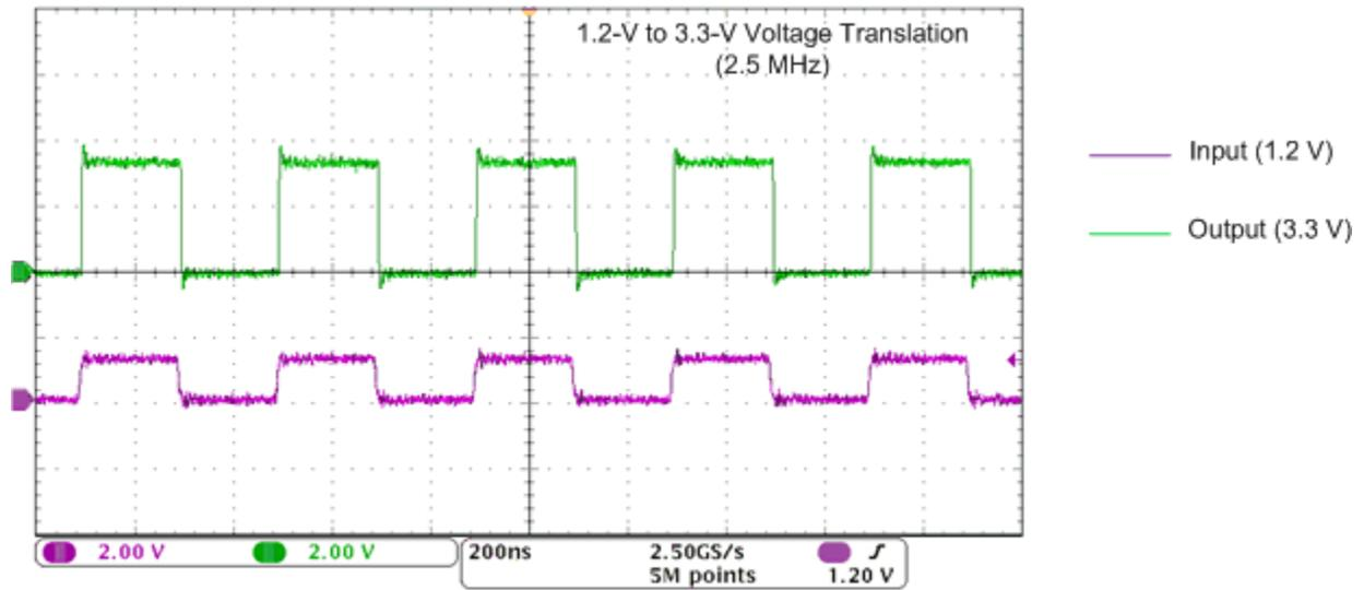
Figure 9-4. Translation Up (1.2V to 3.3V) at 2.5MHz
