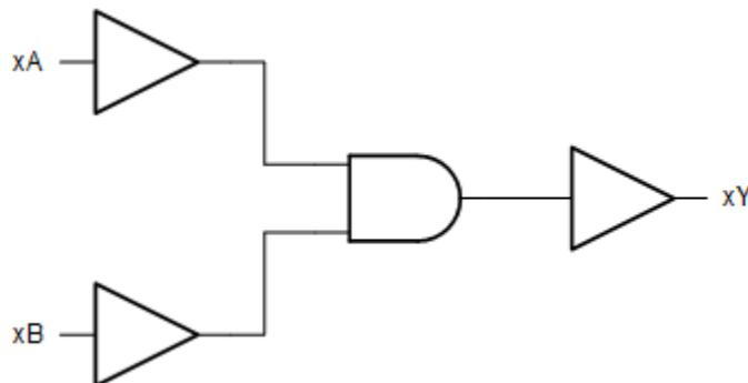
Figure 7-1. Logic Diagram, each gate (Positive Logic)
