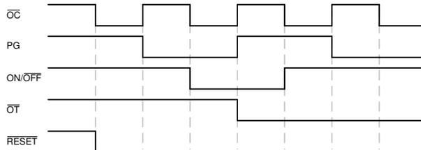
Figure 9-2. Application Timing Diagram
