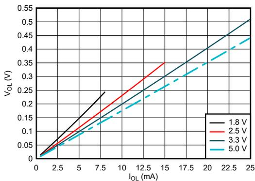
**Figure 6-5. Output Voltage vs Current in LOW State**
