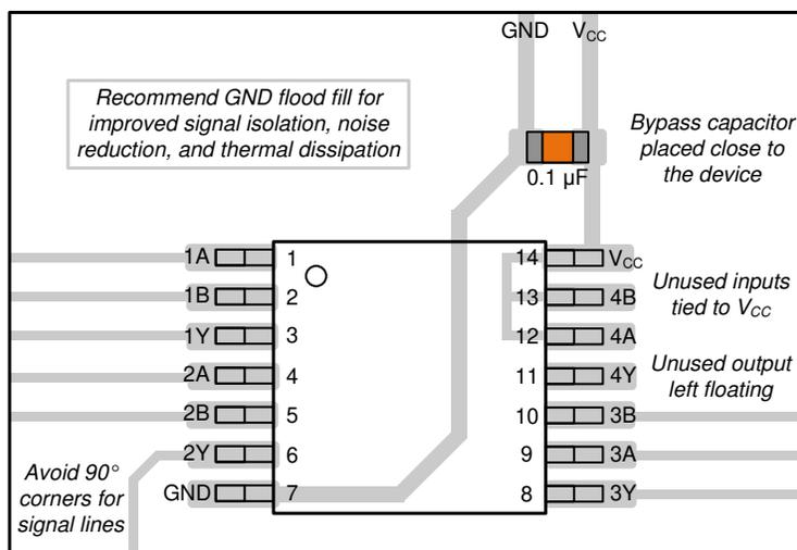
Figure 11-1. Example Layout for the SN74LV4T08
