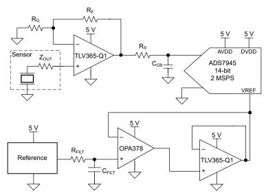
Figure 8-7. TLVx365-Q1 as a SAR ADC Driver
