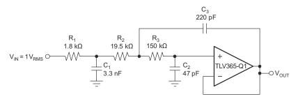
Figure 7-7. Configured as a Three-Pole, 20-kHz, Sallen-Key Filter
