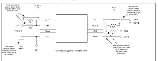
Figure 8-8. Layout Recommendation for TLV2365-Q1 SOIC Package
