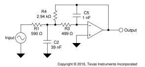
Figure 8-5. Second-Order Low-Pass Filter
