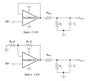
Figure 7-4. Improving Capacitive Load Drive
