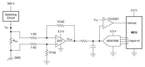
Figure 8-1. Low Side Current Sensing Application Circuit
