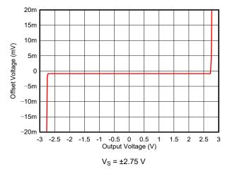
Figure 8-4. Offset Voltage vs Output Swing
