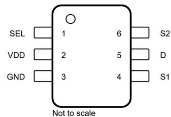
Figure 4-1. DCK Package, 6-Pin SC70 (Top View)
