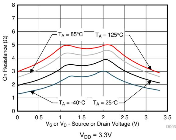
Figure 5-3. On-Resistance vs Temperature
