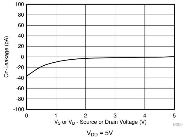
Figure 5-6. On-Leakage vs Source or Drain Voltage
