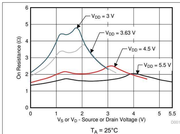
Figure 5-1. On-Resistance vs Source or Drain Voltage
