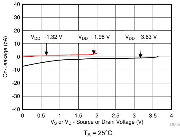
Figure 5-5. On-Leakage vs Source or Drain Voltage
