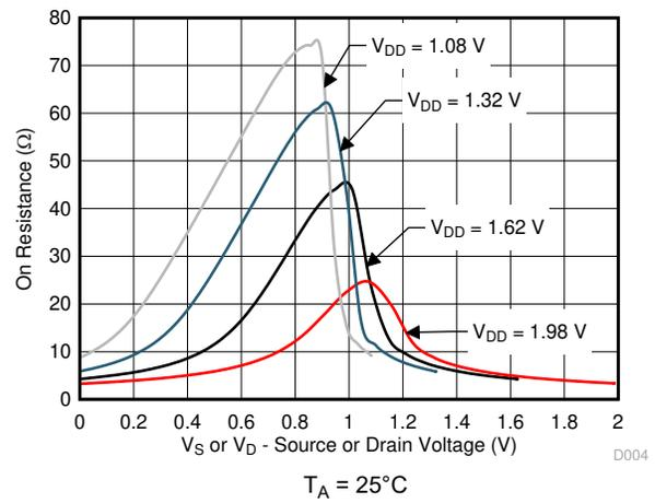
Figure 5-4. On-Resistance vs Source or Drain Voltage
