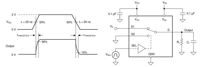
Figure 7-4. Transition-Time Measurement Setup
