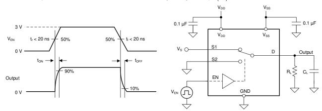
Figure 7-5. Turn-On and Turn-Off Time Measurement Setup
