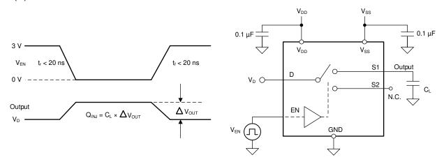
Figure 7-9. Charge-Injection Measurement Setup
