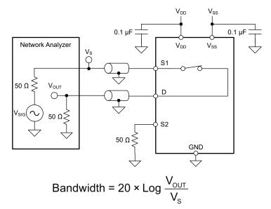
Figure 7-12. Bandwidth Measurement Setup
