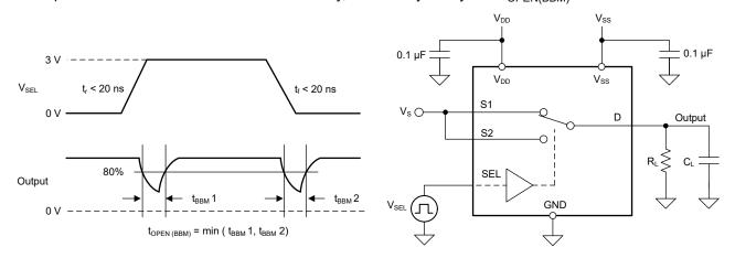
Figure 7-6. Break-Before-Make Delay Measurement Setup
