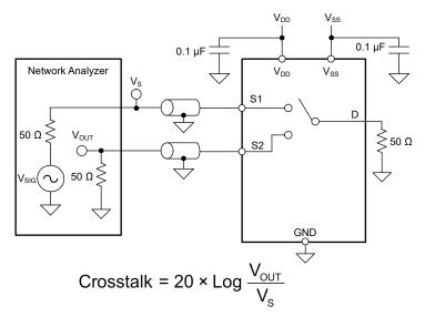
Figure 7-11. Crosstalk Measurement Setup
