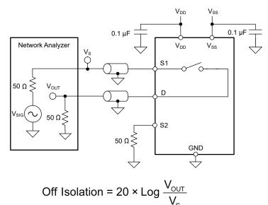
Figure 7-10. Off Isolation Measurement Setup
