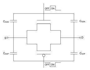
Figure 8-1. Transmission Gate Topology
