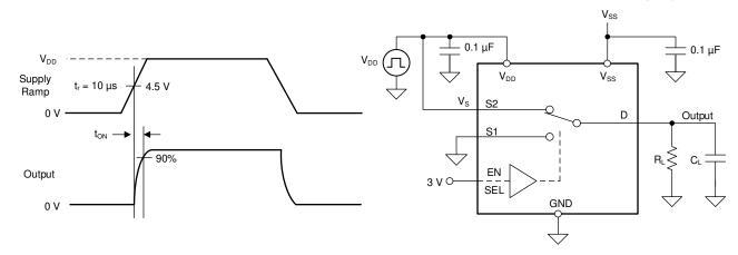
Figure 7-7. t<sub>ON (VDD)</sub> Time Measurement Setup
