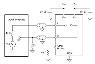
Figure 7-13. THD + N Measurement Setup
