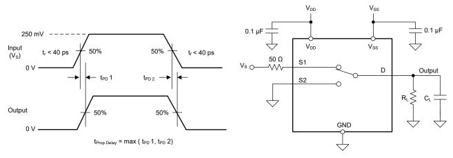
Figure 7-8. Propagation Delay Measurement Setup
