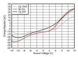
Figure 8-2. Charge Injection Compensation
