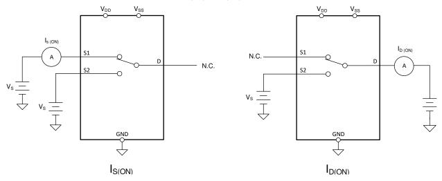
Figure 7-3. On-Leakage Measurement Setup
