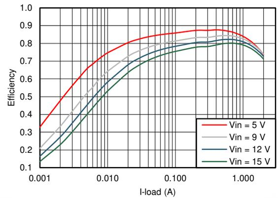
**Figure 7-5. TPS562201 Efficiency,  $V_{OUT} = 1.05\text{ V}$**
