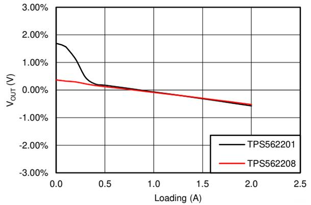
**Figure 7-3. Load Regulation  $V_{IN} = 12\text{ V}$**
