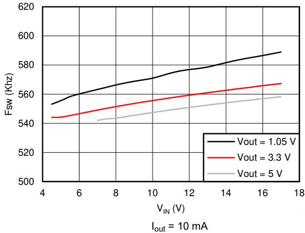
**Figure 5-7. TPS562208 Switching Frequency vs Input Voltage**
