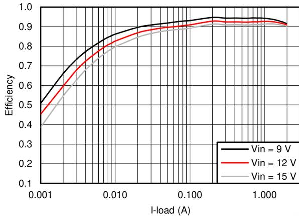
**Figure 5-13. TPS562201  $V_{OUT} = 5\text{ V}$  Efficiency,  $L = 3.3\ \mu\text{H}$**
