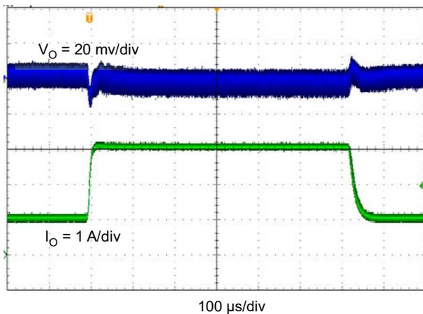
**Figure 7-12. TPS562201 Transient Response, 0.75 to 2.25 A**
