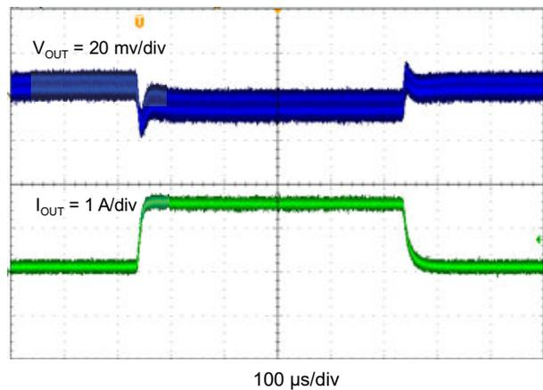
**Figure 7-13. TPS562208 Transient Response 0.1 to 2 A**
