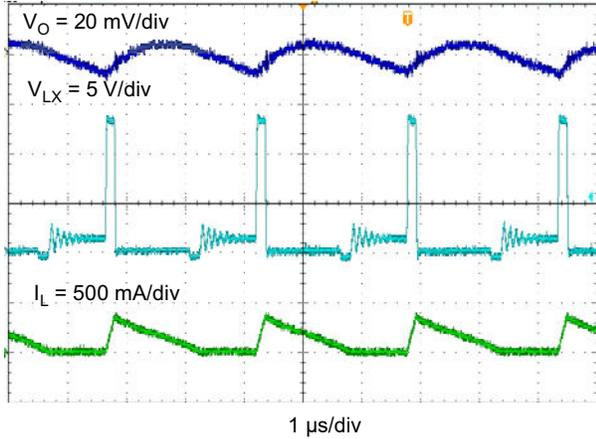
**Figure 7-8. TPS562201 Output Voltage Ripple,  $I_{OUT} = 0.25\text{ A}$**
