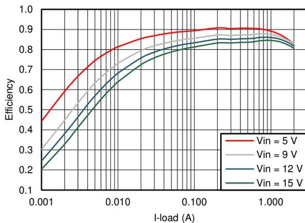
**Figure 5-11. TPS562201  $V_{OUT} = 1.8\text{ V}$  Efficiency,  $L = 2.2\ \mu\text{H}$**
