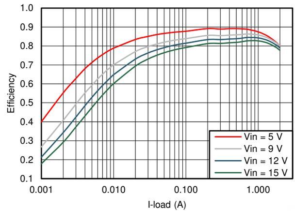
**Figure 5-10. TPS562201  $V_{OUT} = 1.5\text{ V}$  Efficiency,  $L = 2.2\ \mu\text{H}$**
