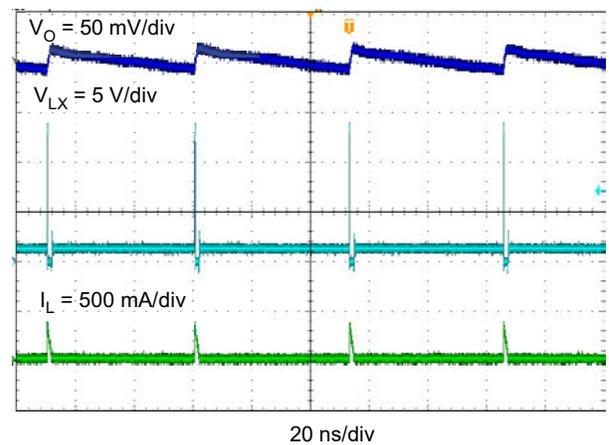
**Figure 7-7. TPS562201 Output Voltage Ripple,  $I_{OUT} = 10\text{ mA}$**
