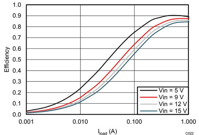
**Figure 5-16. TPS562208  $V_{OUT} = 1.8\text{ V}$  Efficiency,  $L = 2.2\ \mu\text{H}$**
