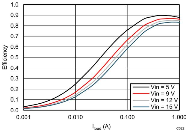
**Figure 5-15. TPS562208  $V_{OUT} = 1.5\text{ V}$  Efficiency,  $L = 2.2\ \mu\text{H}$**
