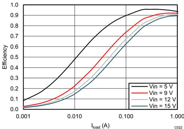
**Figure 5-17. TPS562208  $V_{OUT} = 3.3\text{ V}$  Efficiency,  $L = 2.2\ \mu\text{H}$**
