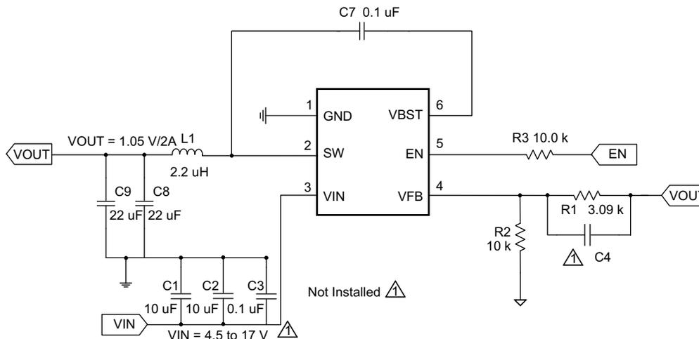
Figure 7-1. TPS562201 and TPS562208 1.05-V/2-A Reference Design
