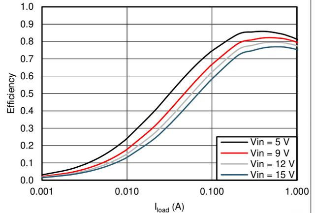
**Figure 5-14. TPS562208  $V_{OUT} = 1.05\text{ V}$  Efficiency,  $L = 2.2\ \mu\text{H}$**
