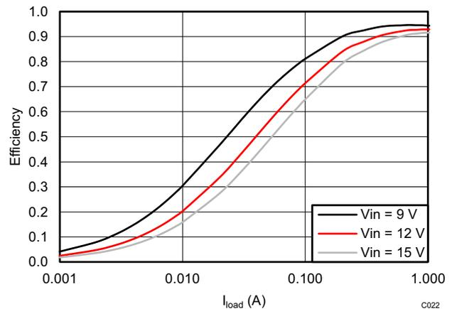
**Figure 5-18. TPS562208  $V_{OUT} = 5\text{ V}$  Efficiency,  $L = 3.3\ \mu\text{H}$**
