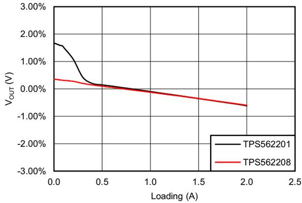
**Figure 7-2. Load Regulation,  $V_{IN} = 5\text{ V}$**
