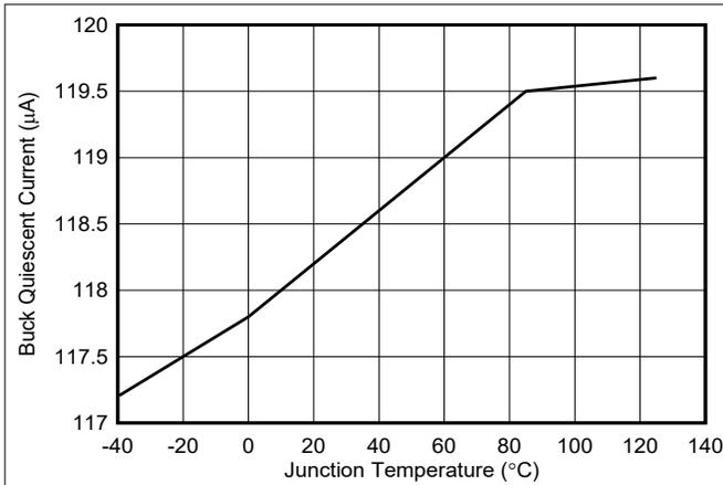
**Figure 5-1. TPS562201 Supply Current vs Junction Temperature**
