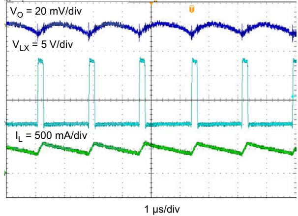
**Figure 7-9. TPS562201 Output Voltage Ripple,  $I_{OUT} = 2\text{ A}$**
