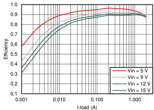
**Figure 5-12. TPS562201  $V_{OUT} = 3.3\text{ V}$  Efficiency,  $L = 3.3\ \mu\text{H}$**
