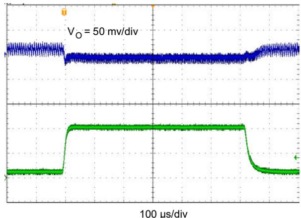
**Figure 7-11. TPS562201 Transient Response, 0.1 to 1.5 A**
