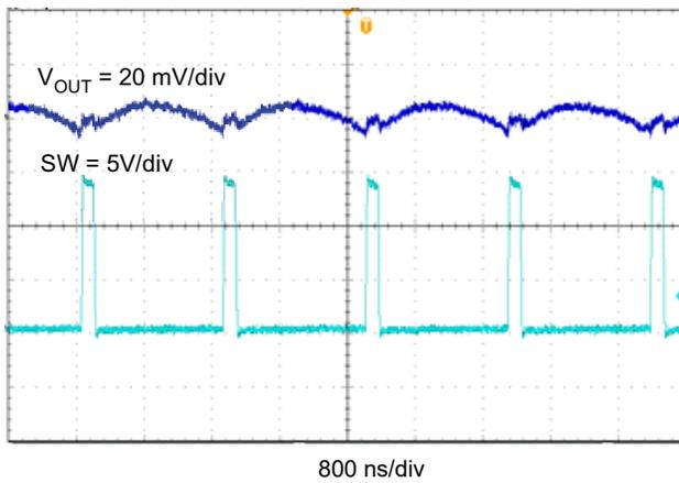
**Figure 7-10. TPS562208 Output Voltage Ripple,  $I_{OUT} = 0\text{ A}$**
