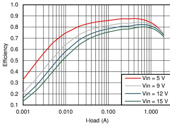
**Figure 5-9. TPS562201  $V_{OUT} = 1.05\text{ V}$  Efficiency,  $L = 2.2\ \mu\text{H}$**
