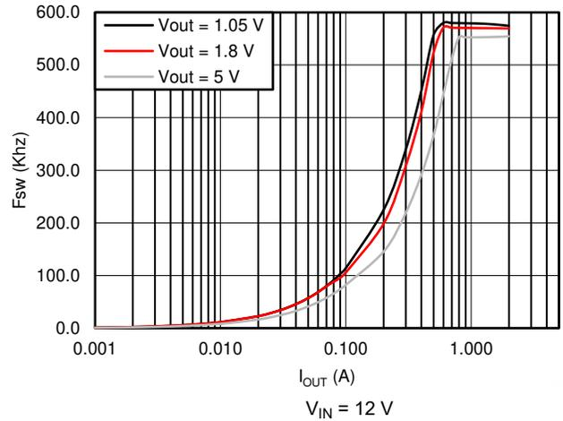
**Figure 5-8. TPS562201 Switching Frequency vs Output Current**
