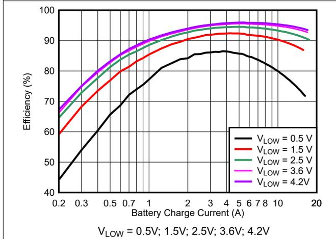
Figure 5-3. Efficiency  $V_{HIGH} = 15\text{ V}$  Buck Mode
