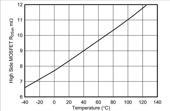
Figure 5-6.  $R_{DS(on)}$  vs Temperature
