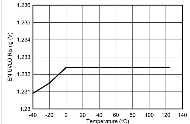
Figure 5-5. EN/UVLO Rising Voltage vs Temperature
