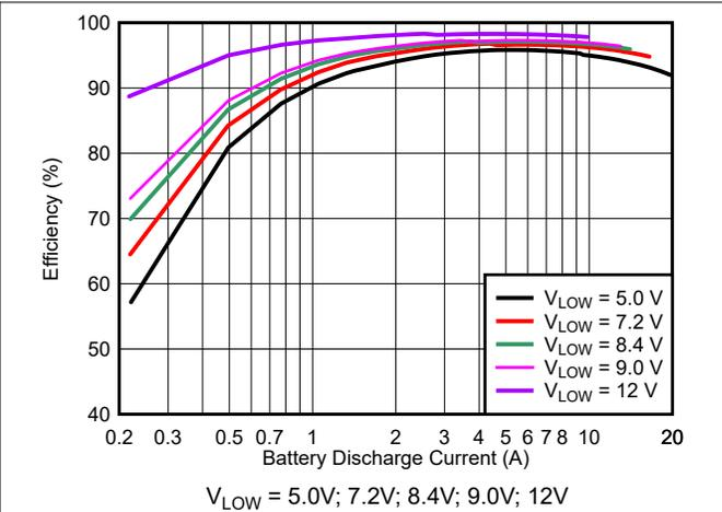
Figure 5-2. Efficiency  $V_{HIGH} = 15\text{ V}$  Boost Mode
