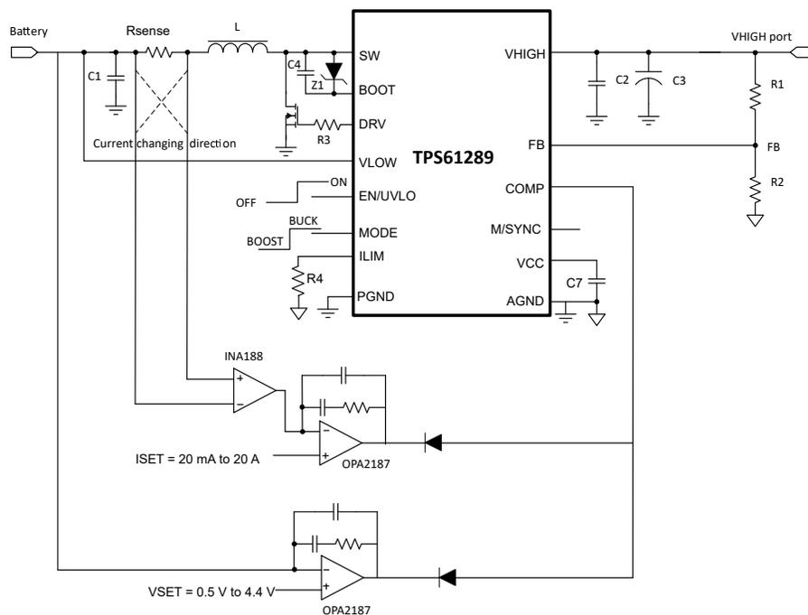
Figure 7-1. TPS61289 Battery Test System Simplified Schematic
