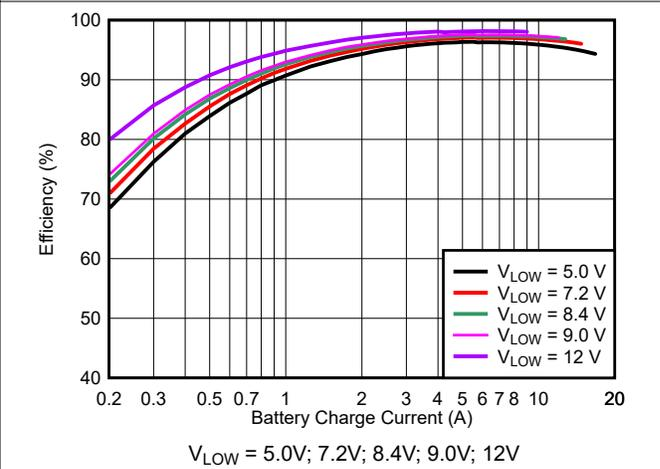
Figure 5-4. Efficiency  $V_{HIGH} = 15\text{ V}$  Buck Mode
