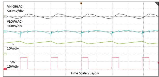
$V_{LOW} = 3.6V$       $V_{HIGH} = 15V$       $I_{Discharge} = 15A$
