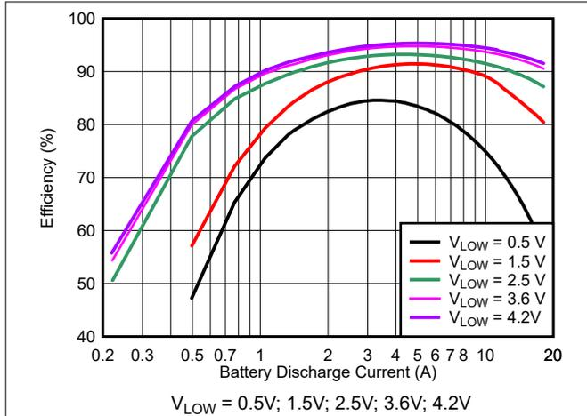
Figure 5-1. Efficiency  $V_{HIGH} = 15\text{ V}$  Boost Mode
