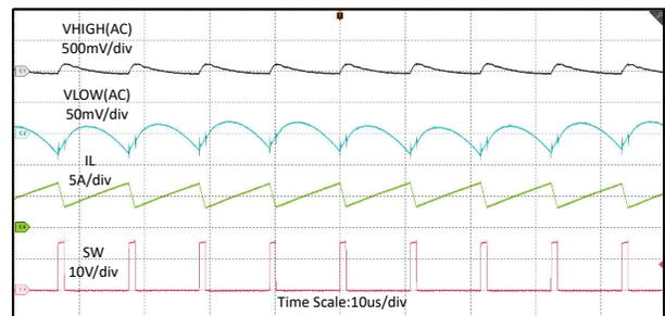
$V_{LOW} = 1.5V$       $V_{HIGH} = 15V$       $I_{Discharge} = 5A$
