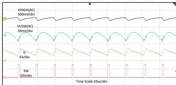
$V_{LOW} = 1.5V$       $V_{HIGH} = 15V$       $I_{Charge} = 5A$
