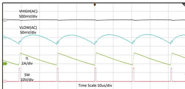
$V_{LOW} = 0.5V$       $V_{HIGH} = 15V$       $I_{Charge} = 1.0A$
