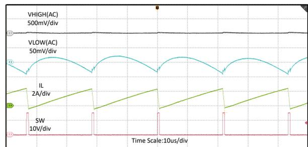
$V_{LOW} = 0.5V$       $V_{HIGH} = 15V$       $I_{Discharge} = 1.0A$
