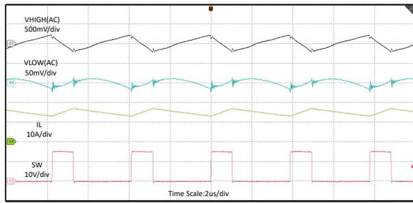
$V_{LOW} = 3.6V$       $V_{HIGH} = 15V$       $I_{Charge} = 15A$
