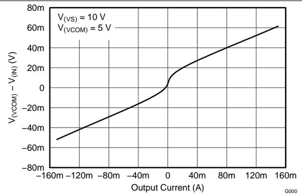
Figure 33. VCOM Buffer Load Regulation
