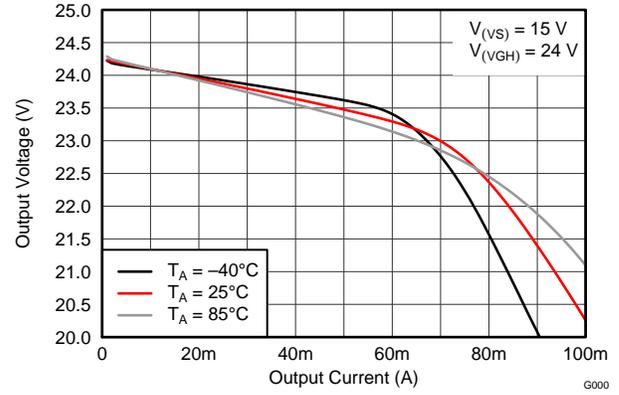
Figure 31. Positive Charge Pump Load Regulation (x2)
