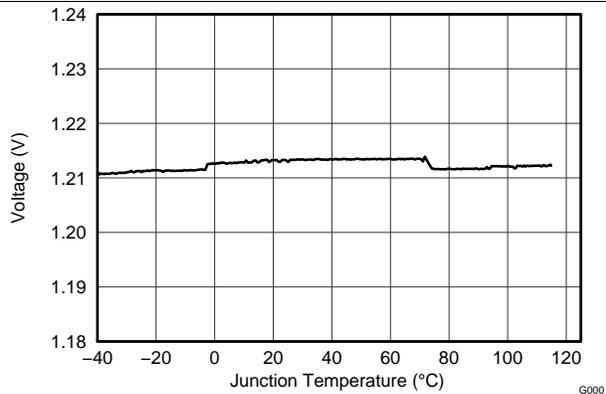
Figure 5. Positive Charge Pump Reference Voltage vs Temperature
