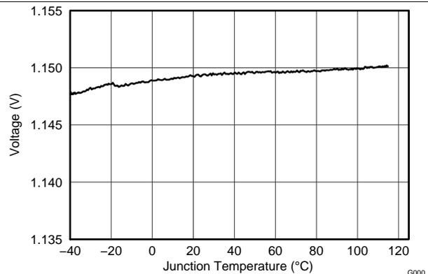
**Figure 4. Boost Converter Reference Voltage vs Temperature**
