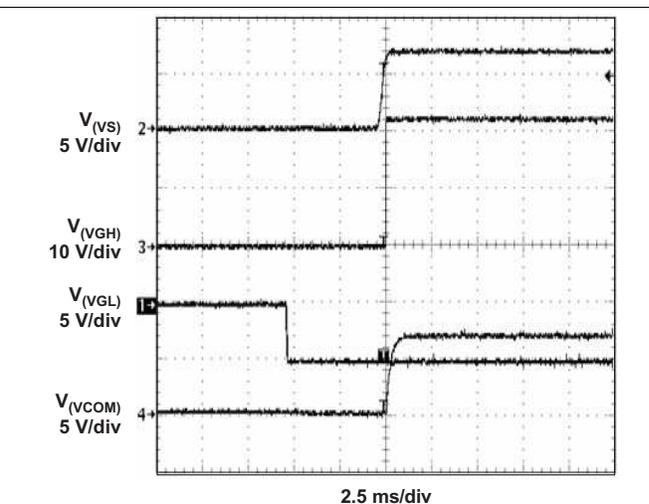
Figure 27. Power-On Sequencing With External Isolation MOSFET
