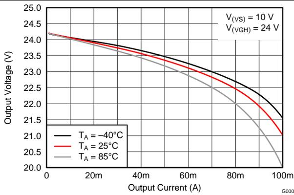
Figure 32. Positive Charge Pump Load Regulation (x3)
