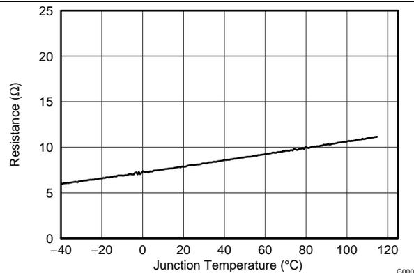
**Figure 3. Boost Converter Rectifier (Q2)  $r_{DS(on)}$  vs Temperature**
