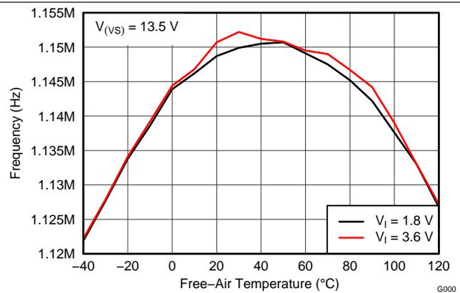
Figure 21. Boost Converter Switching Frequency
