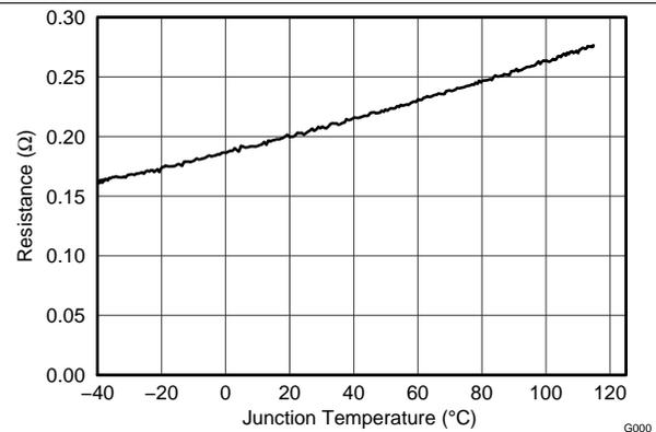
**Figure 2. Boost Converter Switch (Q1)  $r_{DS(on)}$  vs Temperature**
