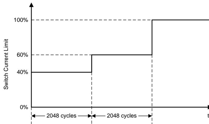
**Figure 9. Boost Converter Switch Current Limit During Soft-Start**
