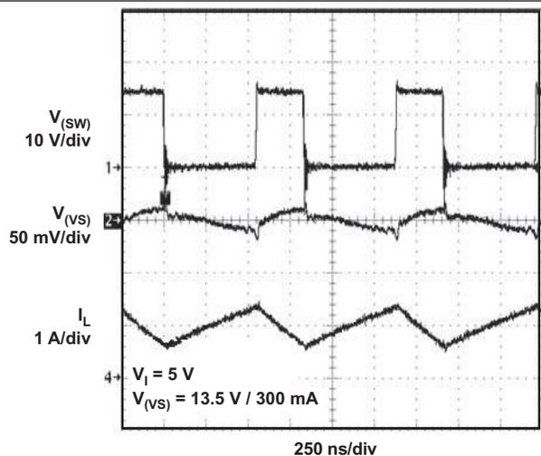
Figure 22. Boost Converter Operation (Nominal Load)
