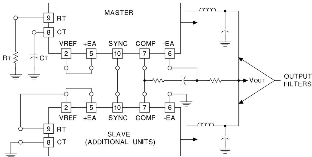
Slaving allows parallel operation of two or more units with equal current sharing.
