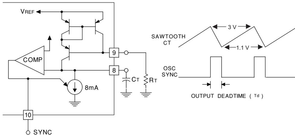
Figure 7. Oscillator Circuit
