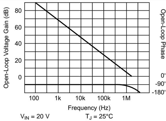
**Figure 8. Error Amplifier Gain and Phase vs Frequency**
