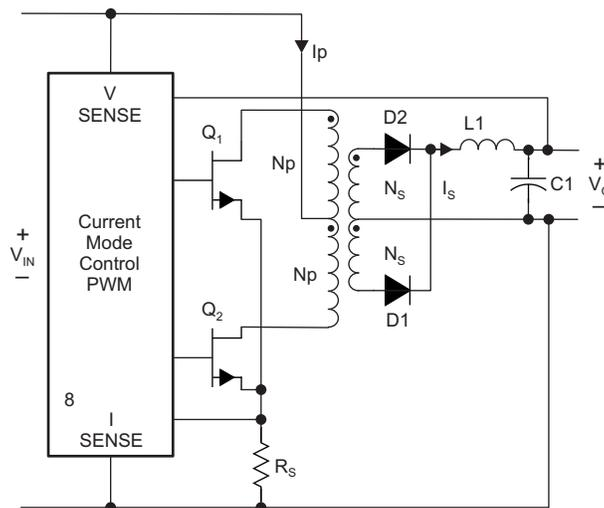
Figure 2. Push-Pull Converter Using Current Mode Control
