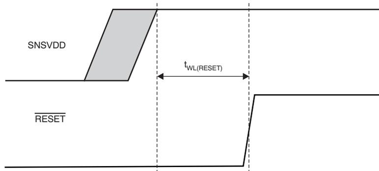
**Figure 4. Recommended Hardware Reset During Power Cycle**
