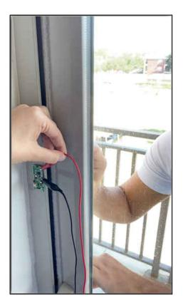
Figure 6-7. Reed Switch Tamper Susceptibility Testing Setup
