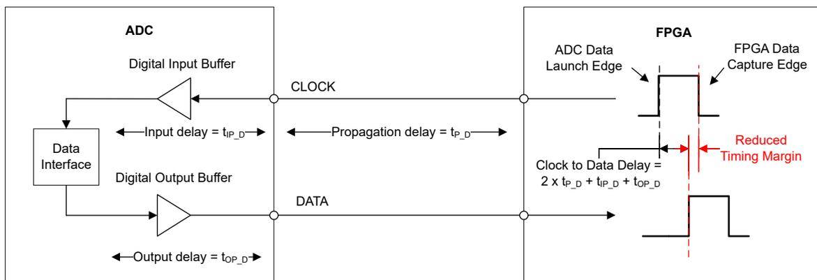
Figure 1. Timing Margin in Regular SPI
