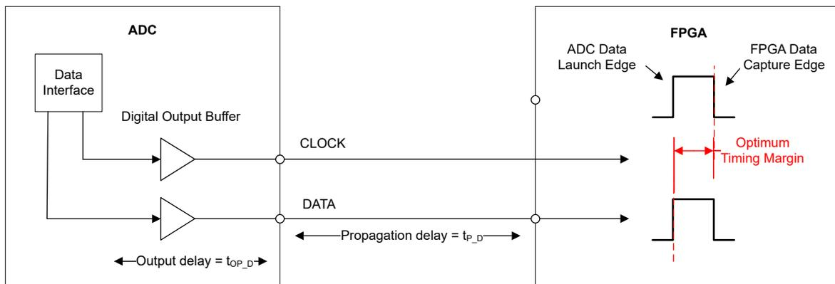
Figure 2. Timing Margin in Source Synchronous Serial Interface
