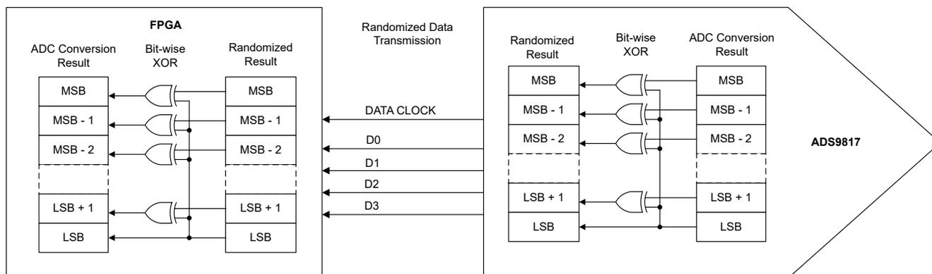
**Figure 3. Bit Scrambling to Reduce Interference Between Data Interference and Analog Performance**
