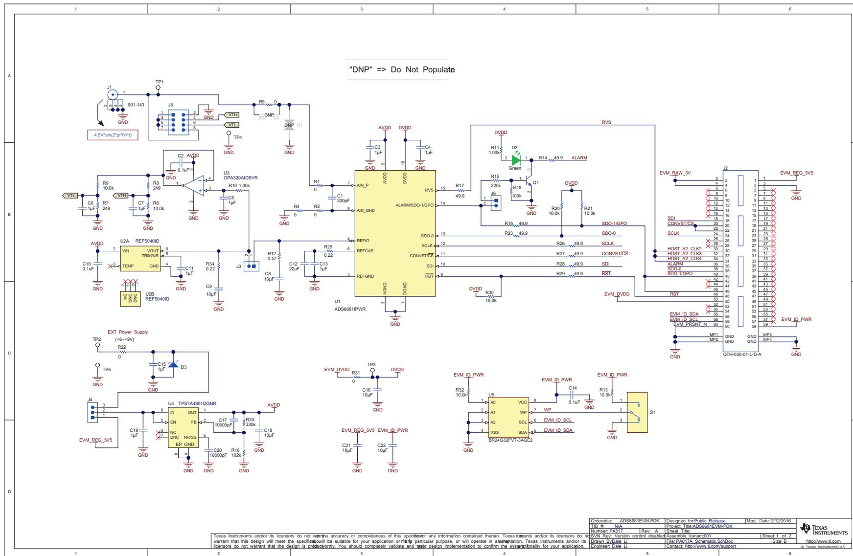
Figure 21. Schematic Diagram of ADS8681EVM – Page 1
