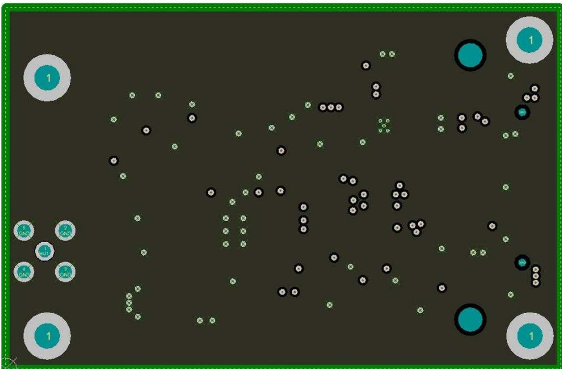
Figure 18. ADS8681EVM PCB Layer 2 – GND Plane
