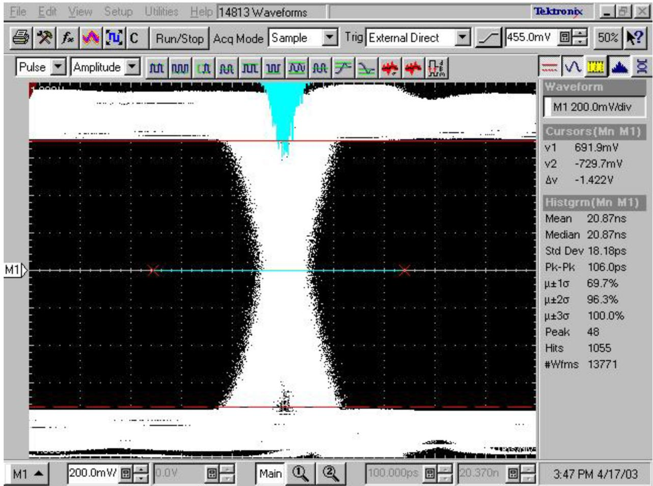
**Figure 5. Zero Crossing of Data Eye at 600 Mbit/sec: R&S
