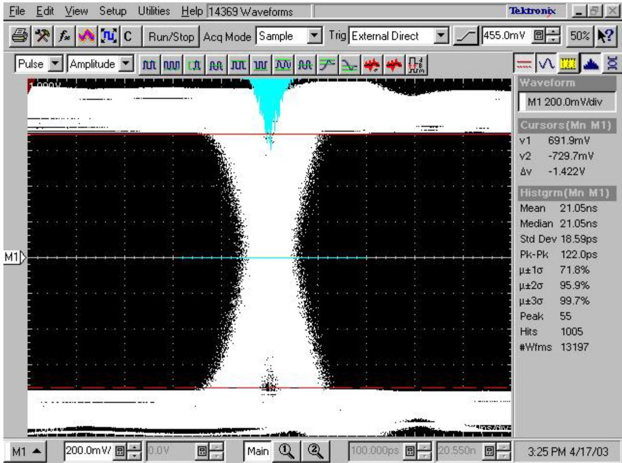
**Figure 6. Zero Crossing of Data Eye at 600 Mbit/sec: R&S SMY02→HP8133A→TLK1501**
