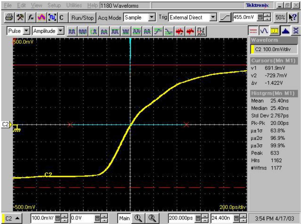
**Figure 3. Zero Crossing of Data Eye at 600 Mbit/sec: R&S SMY02→HP8133A→CDCVF2310 Rising Edge**
