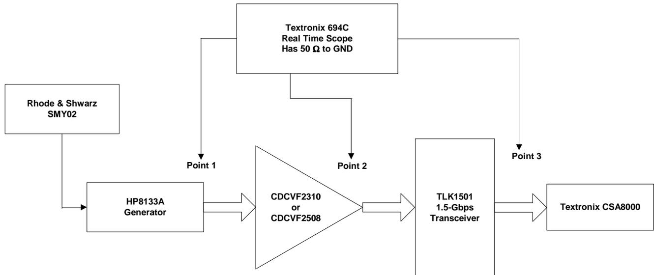
Figure 1. Block Diagram of Test Setup With CDCVF2310 and CDCVF25081 Driving TLK1501
