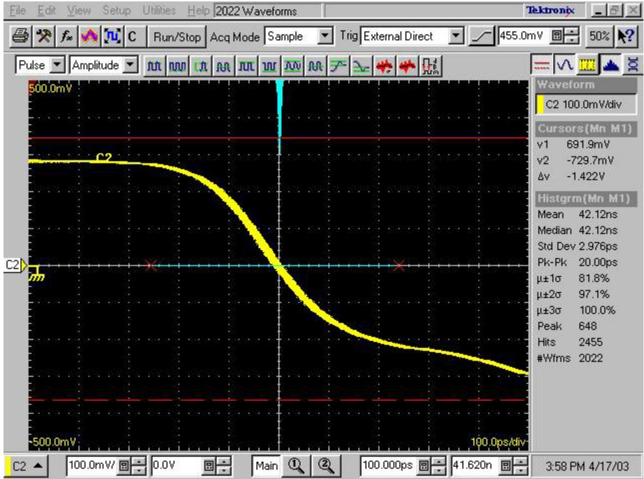
Figure 4. Zero Crossing of Data Eye at 600 Mbit/sec: R&S SMY02→HP8133A→CDCVF2310 Falling Edge
