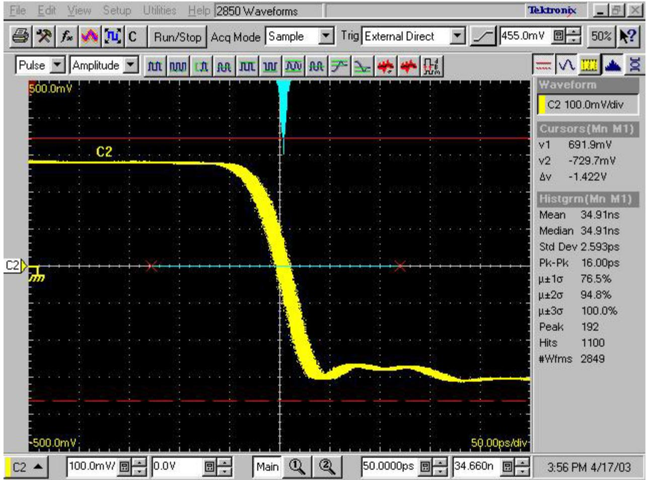
Figure 2. Zero Crossing of Data Eye at 600 Mbit/sec: R&S SMY02→HP8133A
