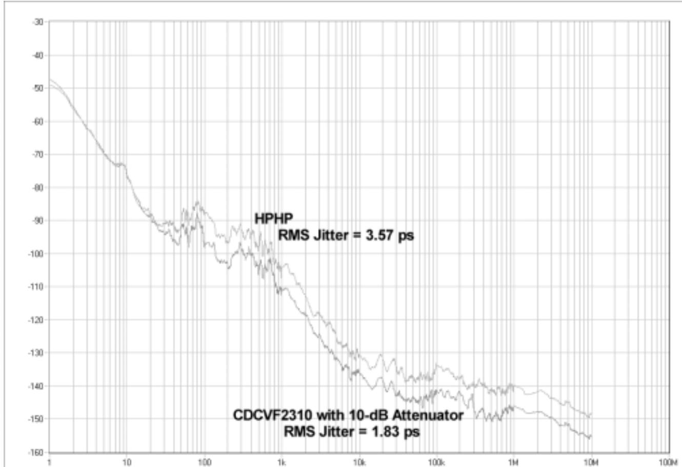
Figure 8. Phase Noise of HP8133A and CDCVF2310 (12 kHz – 10 MHz)
