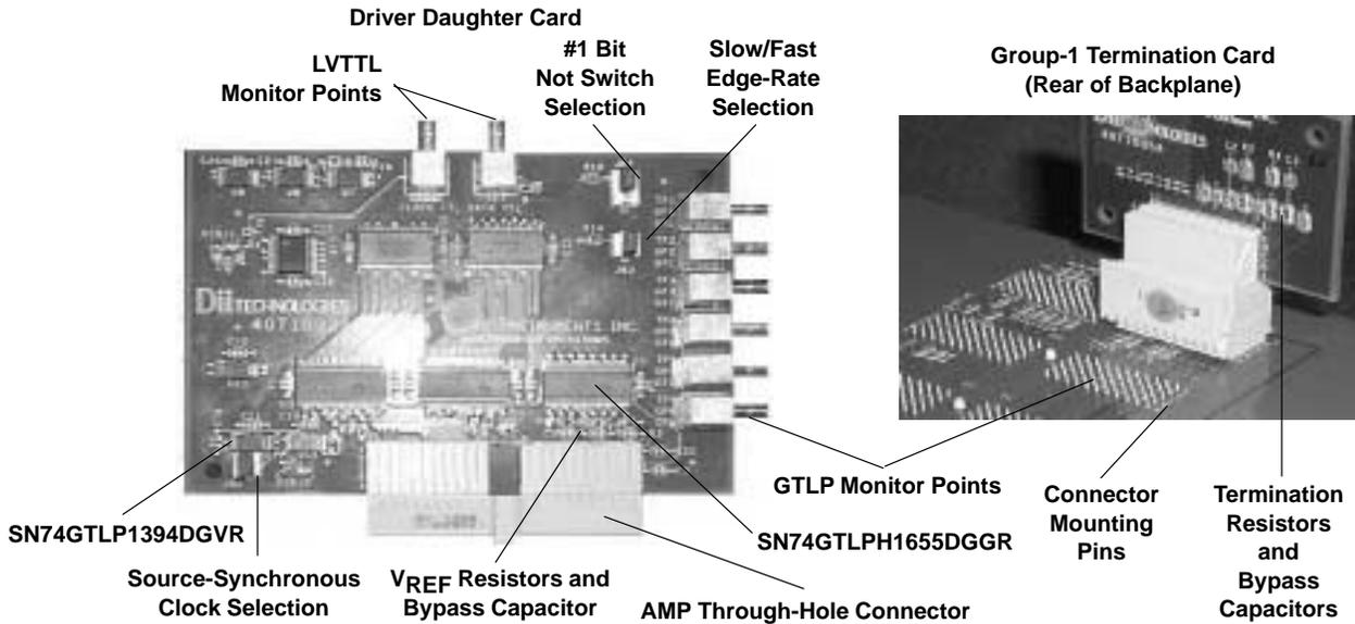
**Figure 7. GTLP EVM Driver and Termination Cards**
