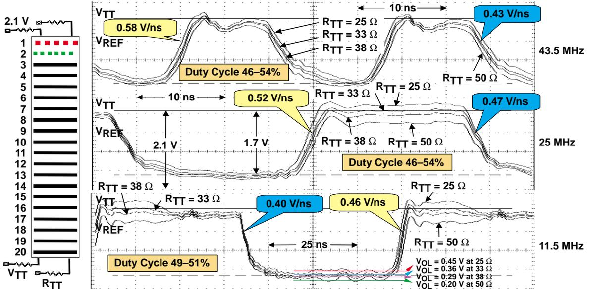
Figure 9. GTLPH1655 Waveforms at BTL Signal Levels (Group 1, Bit 1)
