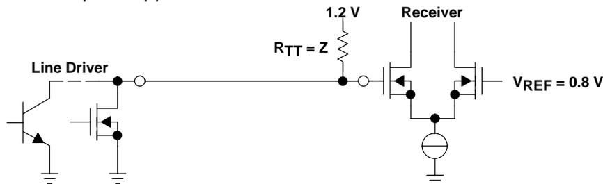
Figure 2. Open-Drain Bus System Using GTL Devices
