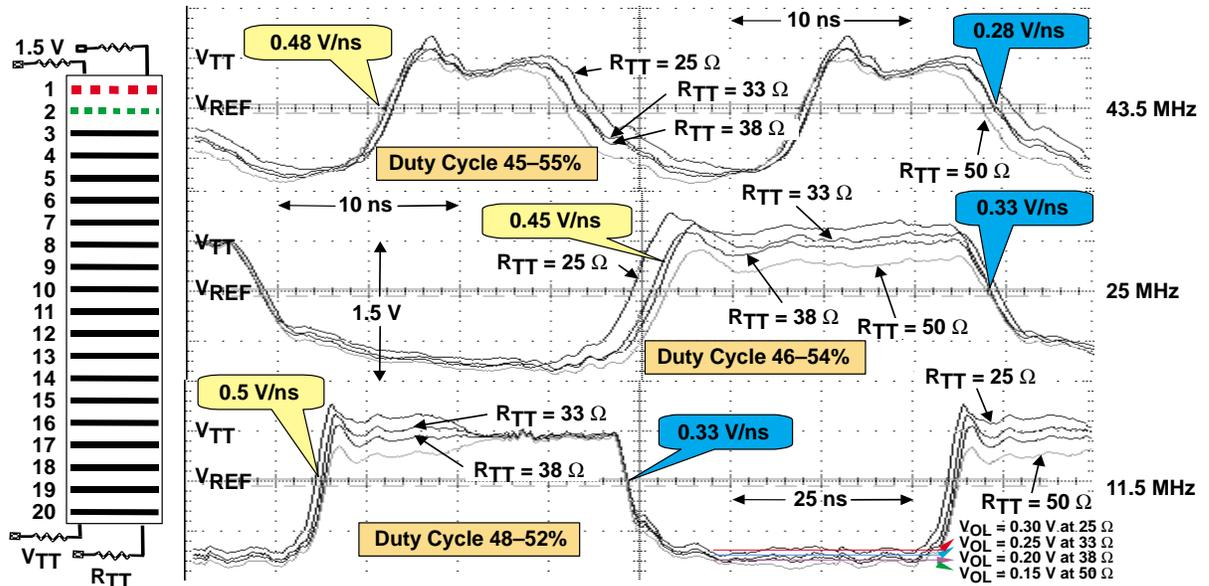
Figure 8. GTLPH1655 Waveforms at GTLP Signal Levels (Group 1, Bit 1)
