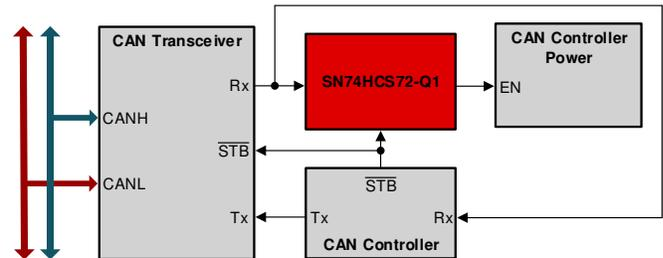
Figure 2. Low Power CAN Wake Solution
