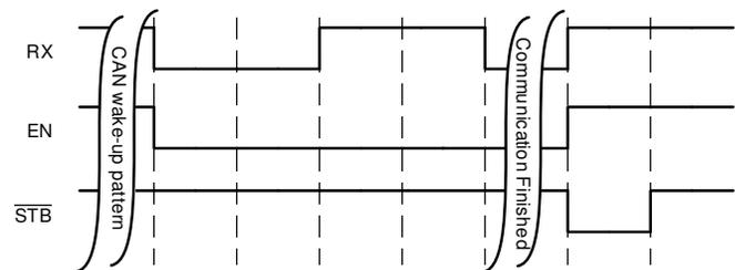
Figure 3. CAN Wake Timing Diagram
