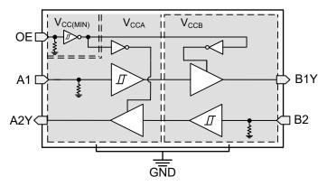
Figure 1-1. Functional Block Diagram
