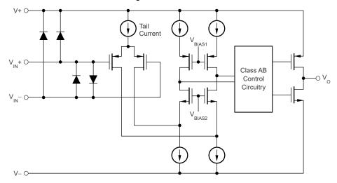
Figure 1-1. Functional Block Diagram
