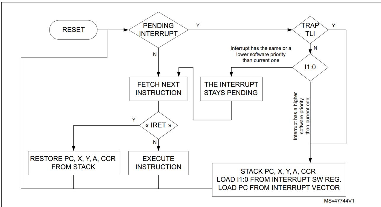
Figure 3-3. Interrupt Processing Flowchart
