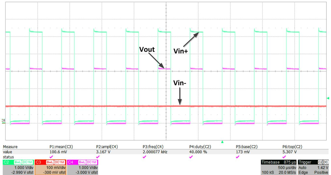
Figure 24. Transient Response of Test Case 1
