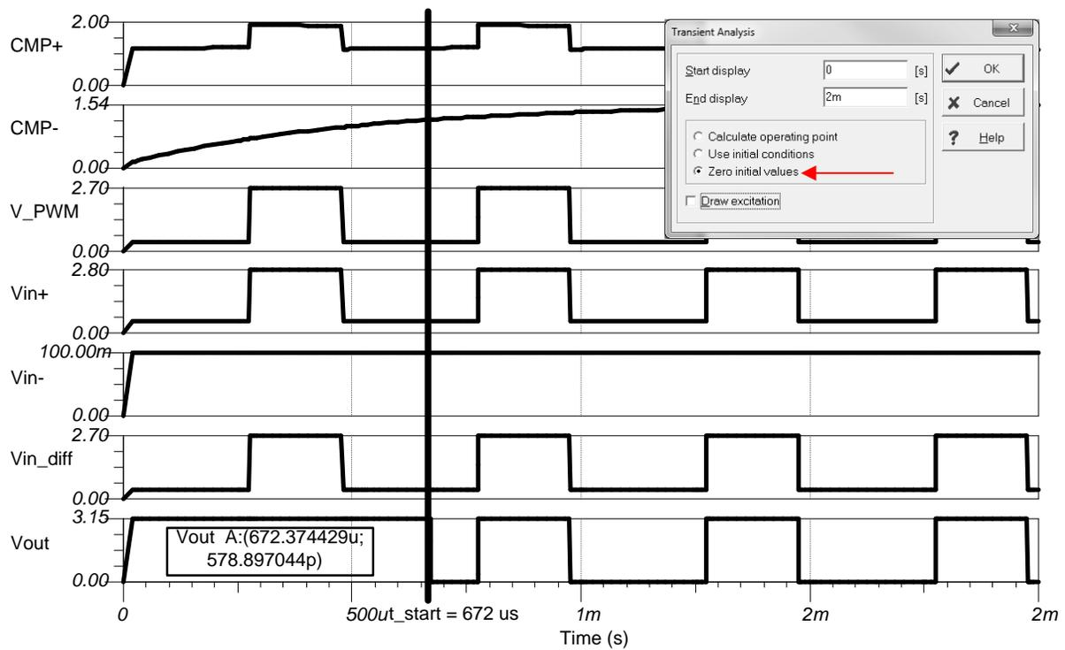
Figure 15. Initial Start Charge Time for CMP-
