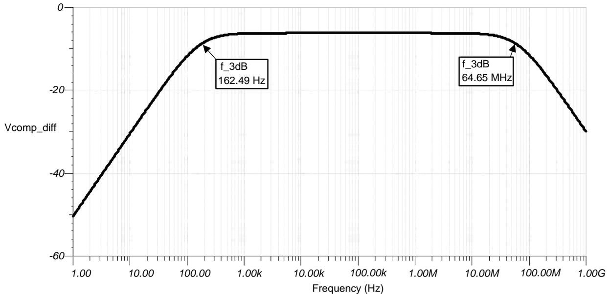
**Figure 10. Input-Scaling Frequency Response**
