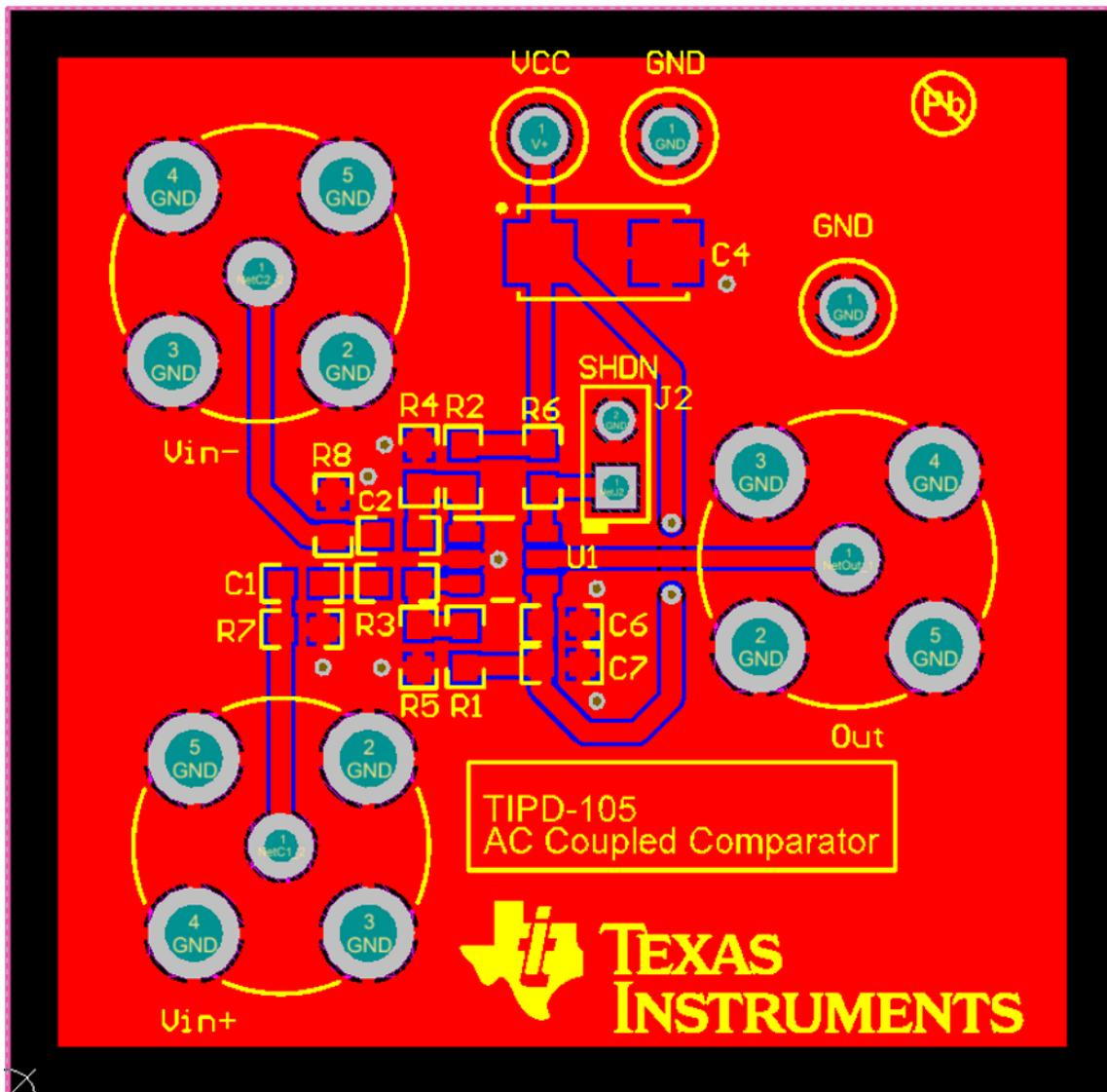
Figure 32. PCB Layout
