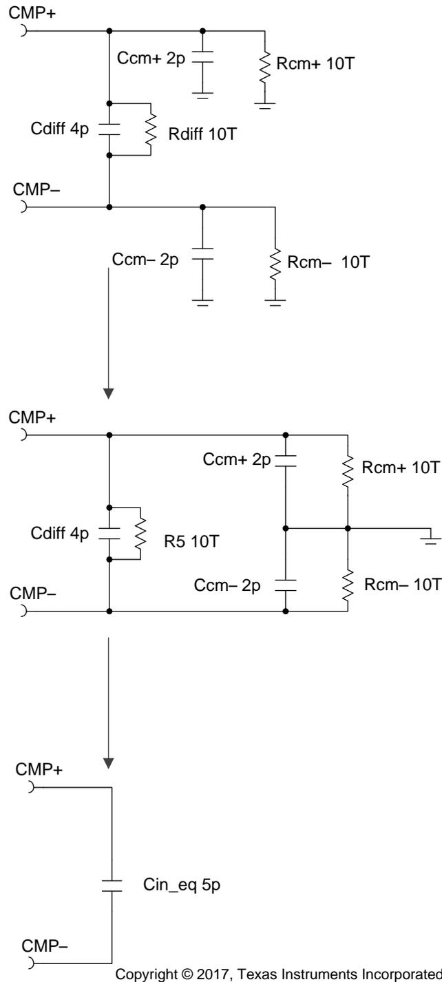
**Figure 4. Comparator Input Capacitance**
