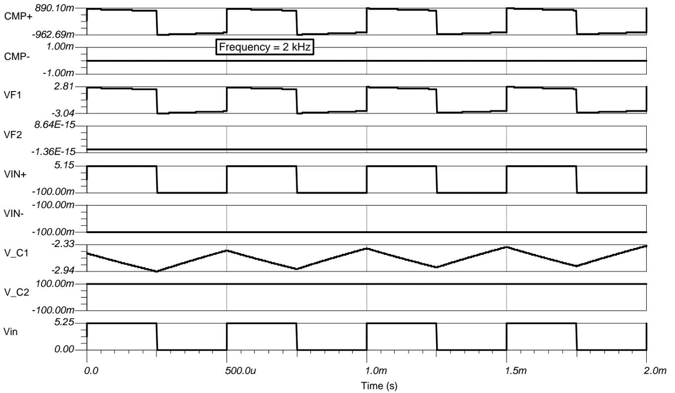
Figure 12. AC-Coupled Signals—Negative Voltage 2 kHz
