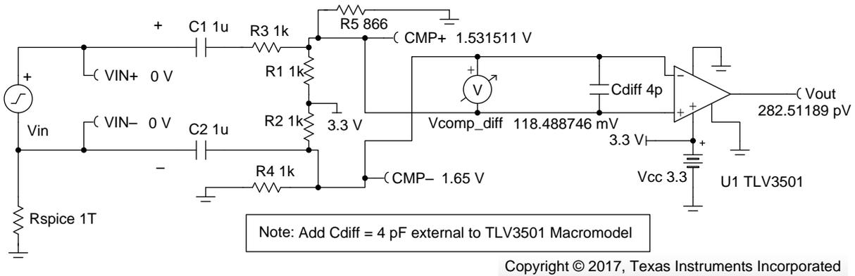
**Figure 9. Input Scaling Frequency Test Circuit**
