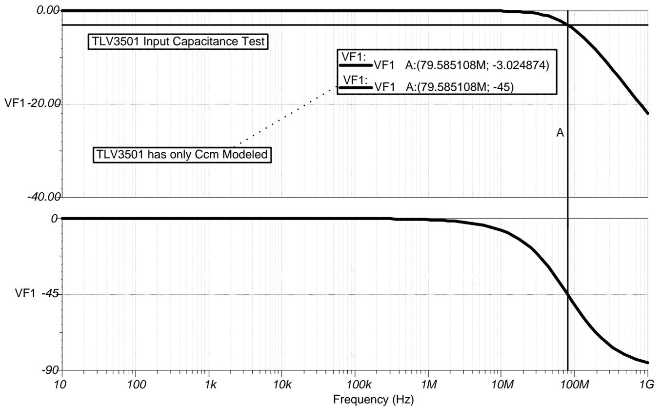
Figure 35. TLV3501 Input Capacitance Simulation Results
