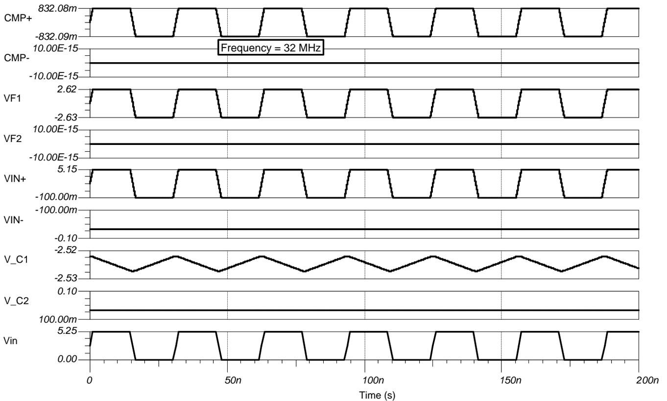
Figure 13. AC-Coupled Signals—Negative Voltage 32 MHz
