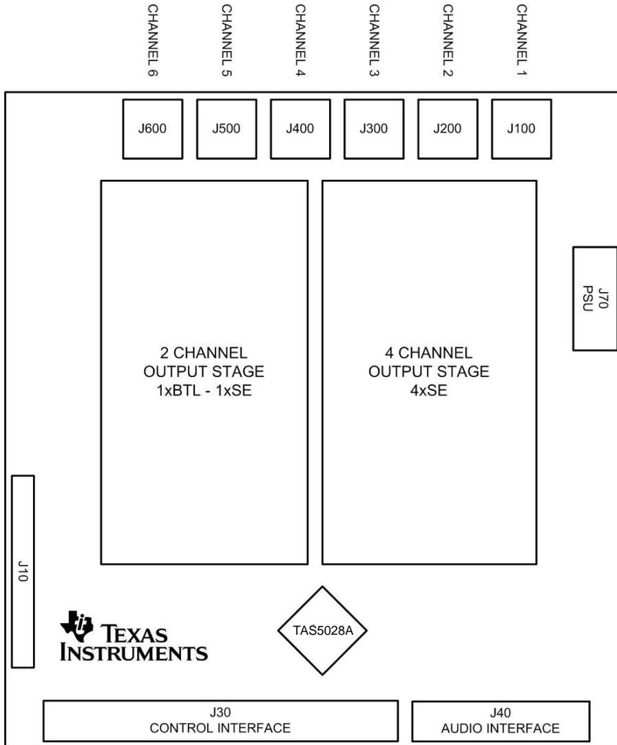
Figure 1-2. Physical Structure for the TAS5028-5122C6EVM (rough outline)
