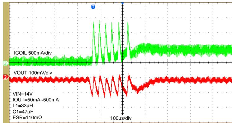
**Figure 2. Load Transient Performance of the TPIC74100EVM**
