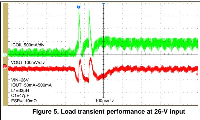
The [Figure 6](#) and [Figure 7](#) show the load transient performance at 33µH and 22µH inductor respectively. With 33µH inductor, the inductor stores more energy before the special circuit exits. The energy causes a little higher overshoot in the VOUT.
