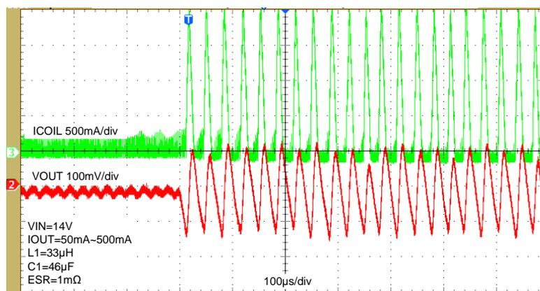
**Figure 3. Load transient performance with ceramic capacitor**
