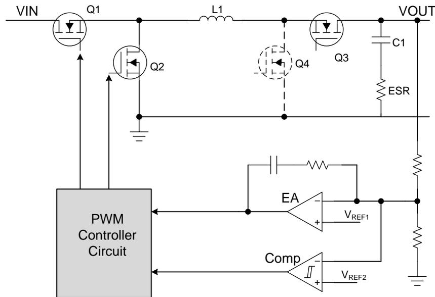
**Figure 1. Simplified Control Circuit of the TPIC74100-Q1**
