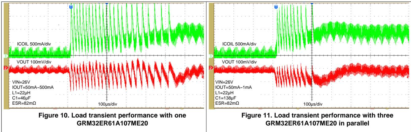
Based on above measurements, following external components are suggested to improve the load transient performance of the TPS74100-Q1.
