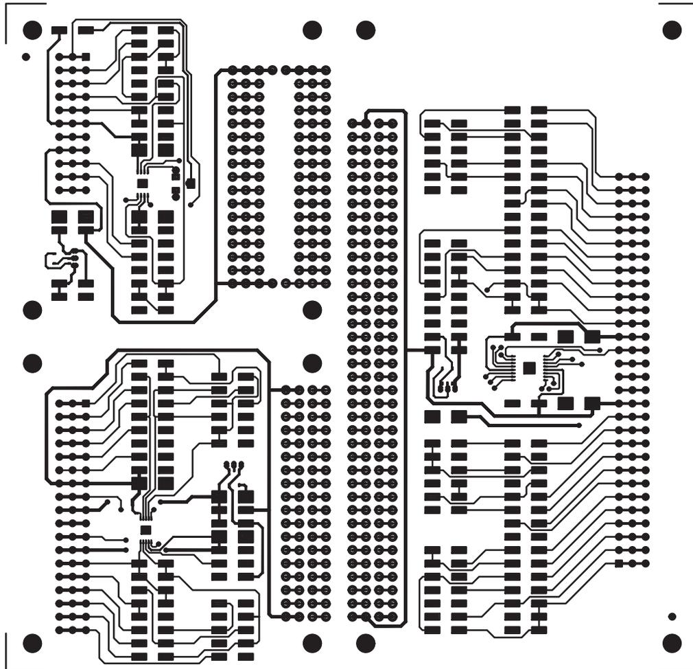
Figure 2–9. EVM Board Layout—Bottom
