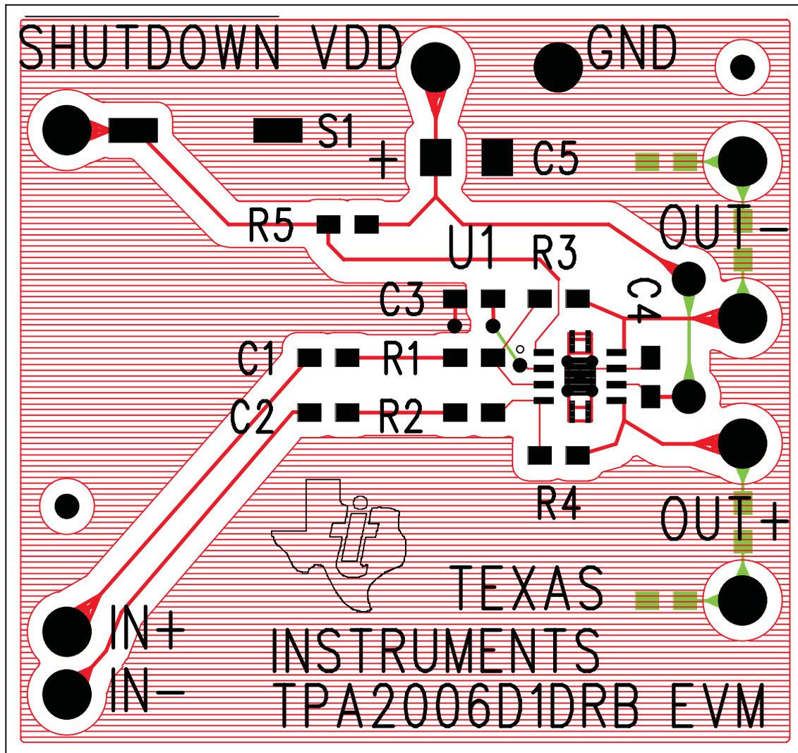
NOTE: Due to the small size of the DRB IC package, the standard part number TPA6002D1DRB is replaced with the code AAOI.
