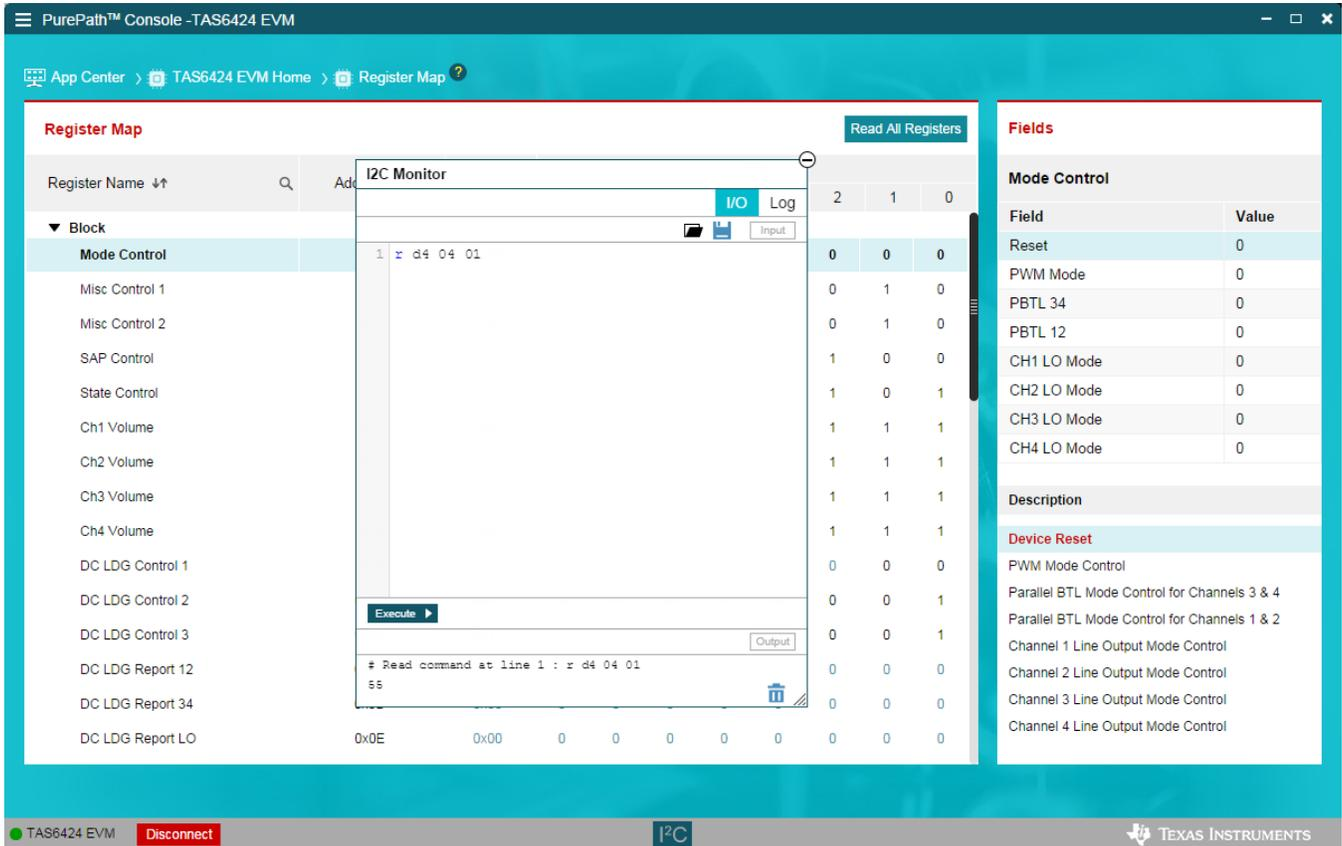
Figure 21. I2C Window – Sending I2C Commands
