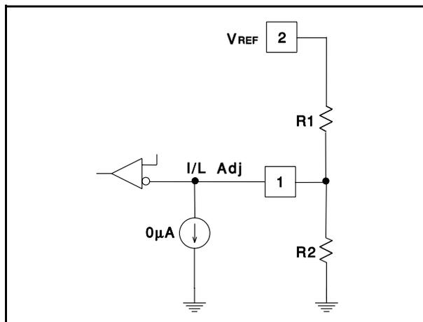
**Figure 2: Superposition with current sink = 0**
