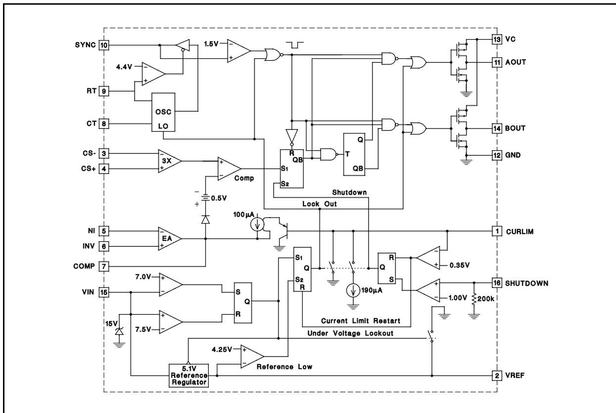
Figure 1: UCC3806 BiCMOS Current Mode PWM Block Diagram
