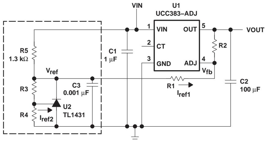
**Figure 2. More Accurate Extended Output Voltage Regulator Schematic**
