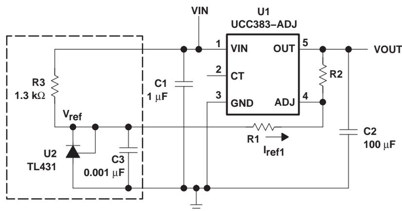
**Figure 1. Extended Output Voltage Regulator Schematic**
