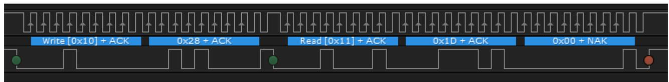
**Figure 1-3. Captured I2C Waveform for Internal Temperature Reading**
