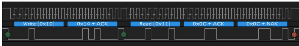
**Figure 1-2. Captured I2C Waveform for Cell 1 Voltage Reading**
