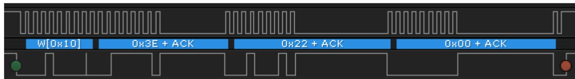
Figure 2-2. Captured I2C Waveform for FET\_ENABLE Subcommand
