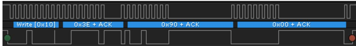
**Figure 3-2. Captured I2C Waveform for SET\_CFGUPATE**
