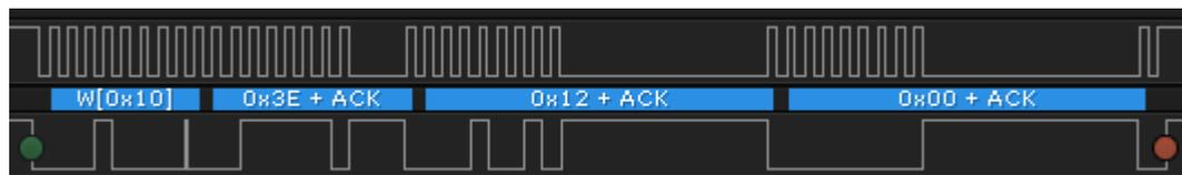
Figure 2-3. Captured I2C Waveform of RESET Subcommand
