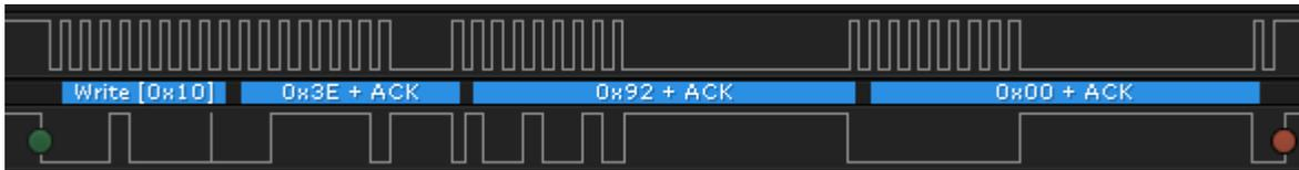
**Figure 3-5. Captured I2C Waveform for EXIT\_CFGUPDATE**
