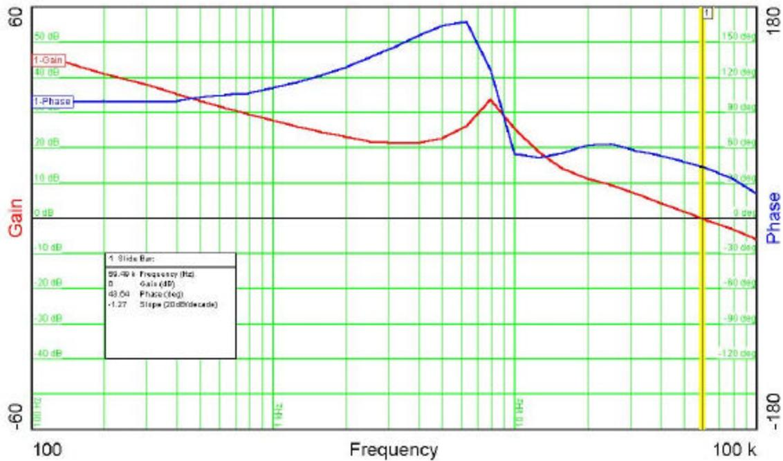
The plot below shows the loop gain and phase margin with output voltage set to 5V. The output was loaded to 6A.  $V_{in} = 12V$
