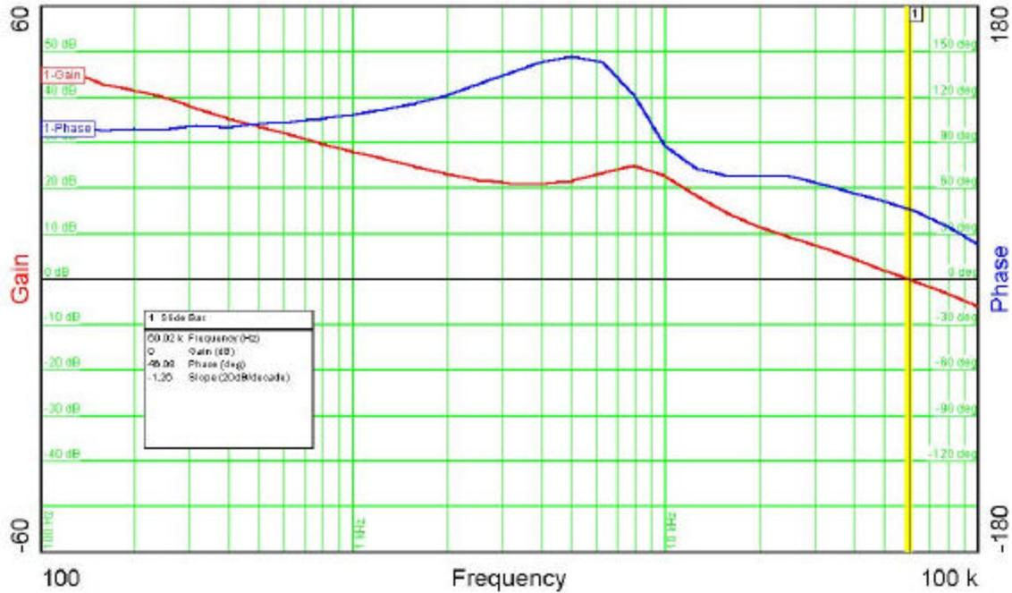
The plot below shows the loop gain and phase margin with output voltage set to 5V. The output was loaded to 3A.  $V_{in} = 12V$
