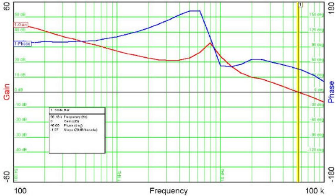
The plot below shows the loop gain and phase margin with output voltage set to 5V. The output shows all 3 variations on one graph.
