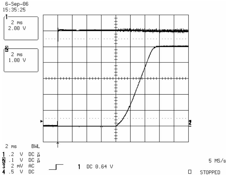
The photo below shows the 5V output voltage (Ch2) startup waveform after the application of 12Vdc in (Ch1). The output was loaded to 6A.
