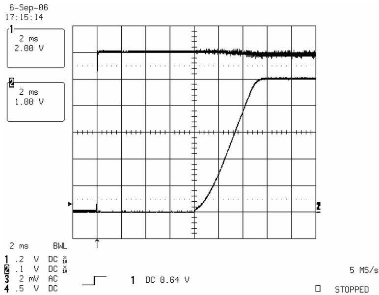
The photo below shows the 5V output voltage (Ch2) shutdown waveform after the removal of 12Vdc in (Ch1). The output was loaded to 6A.
