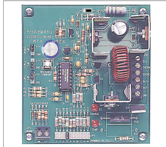
The user provides a power supply and batteries. The user configures the DV2003S2 for the number of cells,  $-\Delta V$  charge termination, and maximum charge time (with or without top-off), and commands the discharge-before-charge option with the push-button switch S1.
