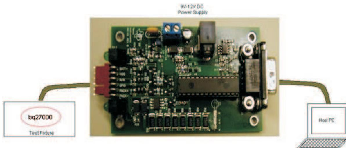
Figure 1. bq27x00 Test and Program Board
