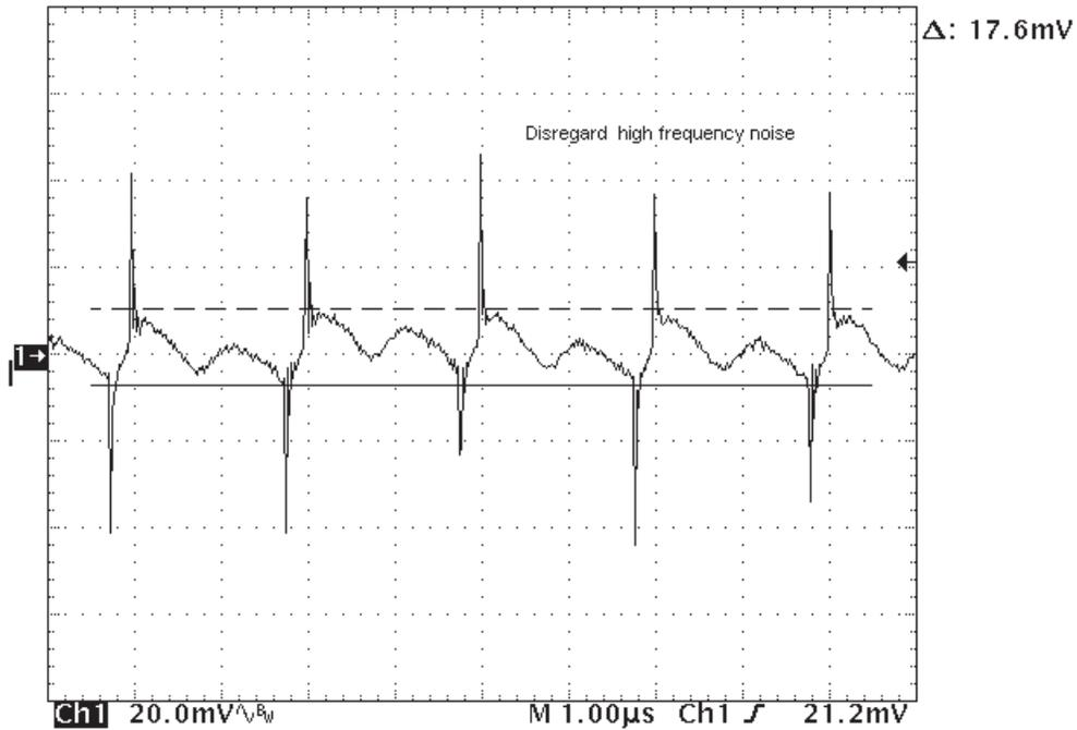
Figure 12. VOUT1 Output Ripple, (VIN = 12 V, IOUT1 = 10 A)
