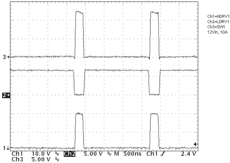
Figure 14. Output 1 Switching waveform, (Ch1 = HDRV1, Ch2 = LDRV1, Ch3 = SW1, VIN = 12 V, I<sub>OUT1</sub> = 10 A)
