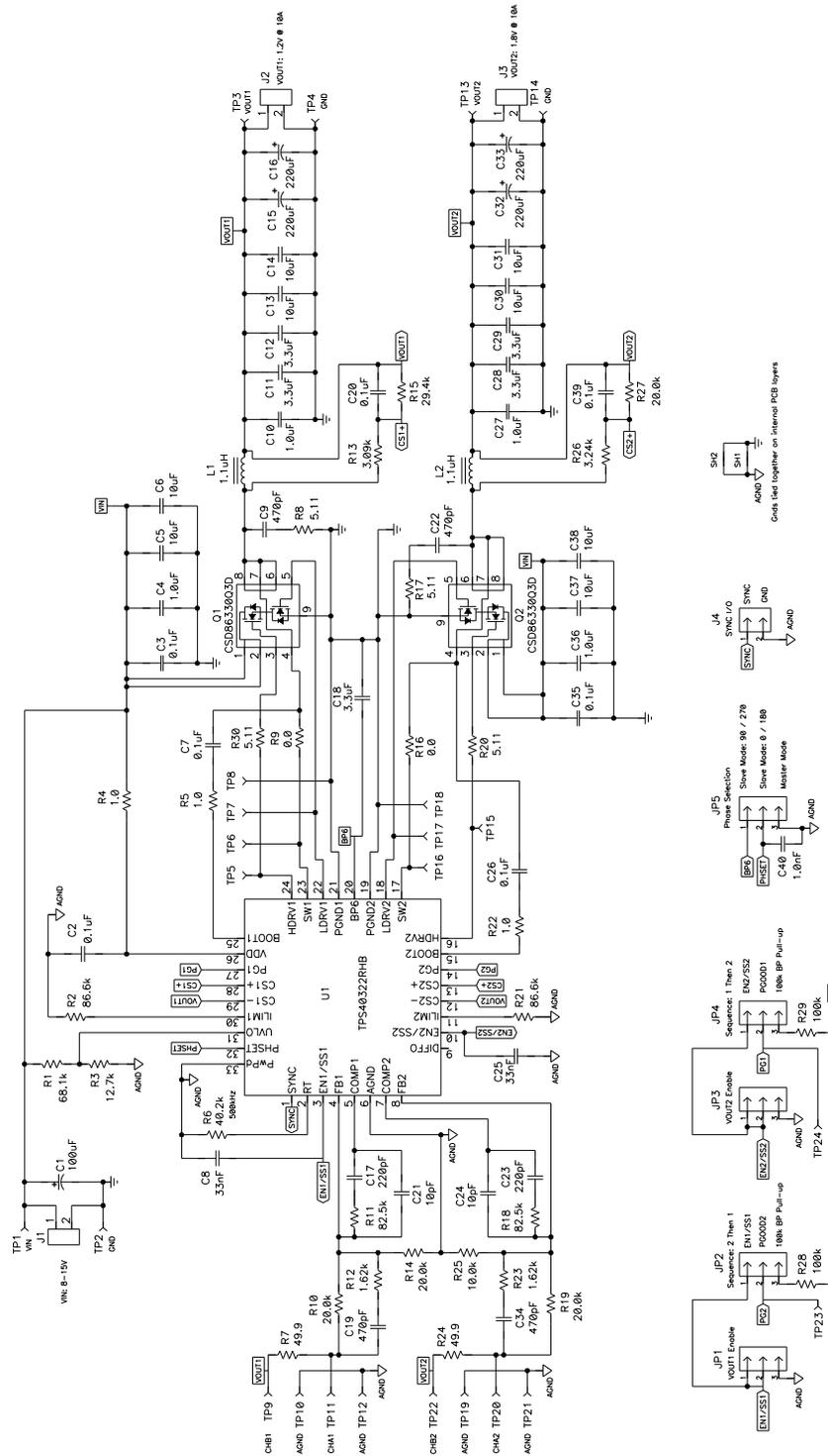
Figure 1. TPS40322EVM-679 Schematic
