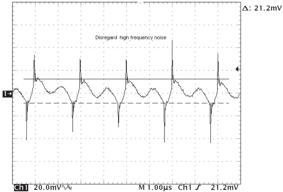
Figure 13. VOUT2 Output Ripple, (VIN = 12 V, IOUT2 = 10 A)
