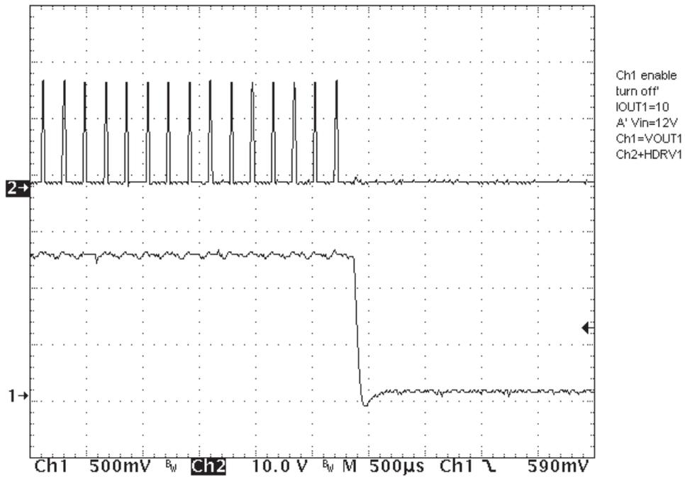
Figure 17. Enable Turn-Off waveform, Ch1 = VOUT1, Ch2 = HDRV1, VIN = 12 V, I<sub>OUT1</sub> = 10 A
