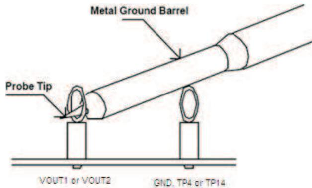
Figure 3. Tip and Barrel Voltage Ripple Measurement
