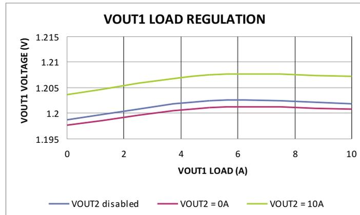
Figure 6. TPS40322EVM-679 VOUT1 Load Regulation, (VIN = 12 V)
