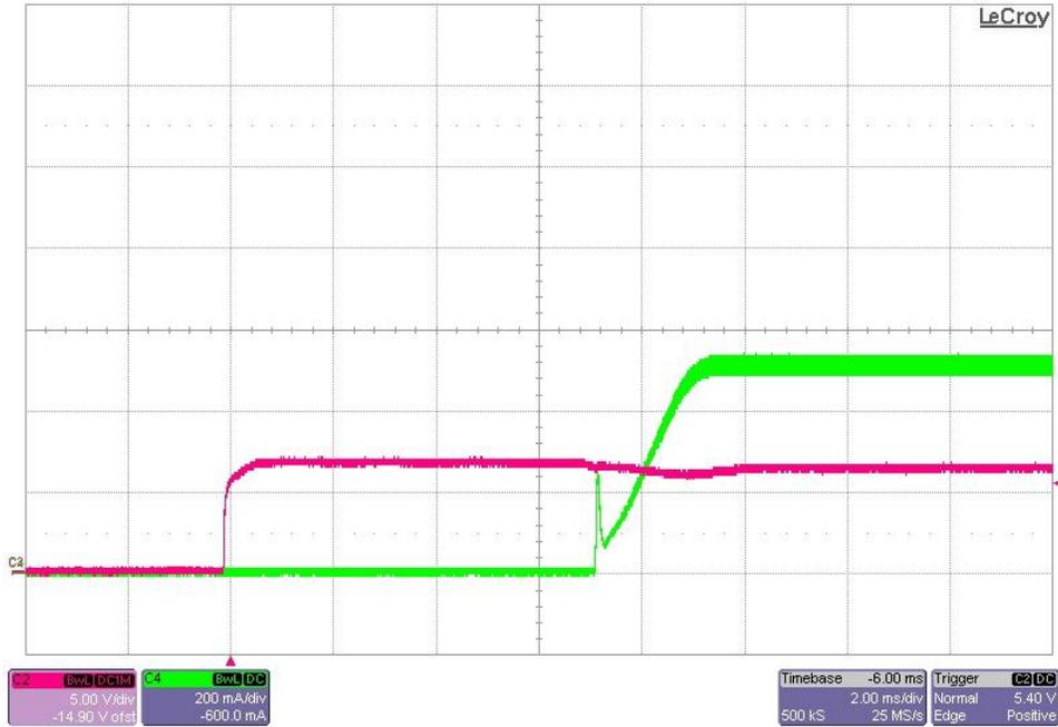
The photo below shows the output current startup waveforms after the application of 12V in. 8 LEDs were used in series and regulated to 0.515A. (5V/DIV, 200mA/DIV, 2mS/DIV)
