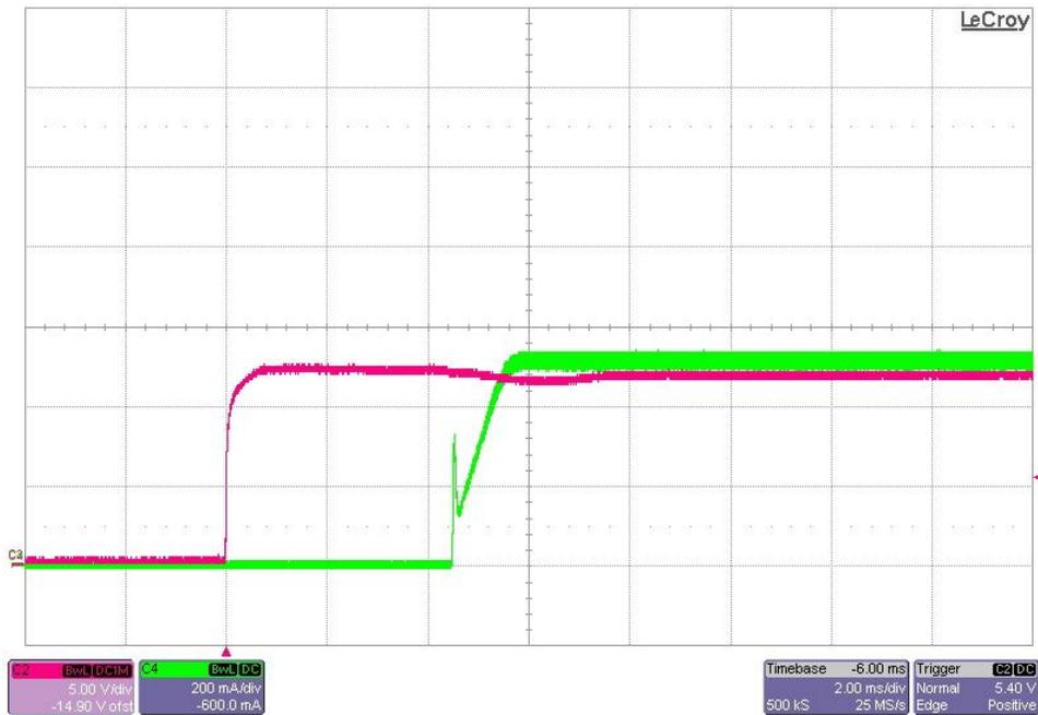
The photo below shows the output current startup waveforms after the application of 36V in. 8 LEDs were used in series and regulated to 0.515A. (10V/DIV, 200mA/DIV, 2mS/DIV)
