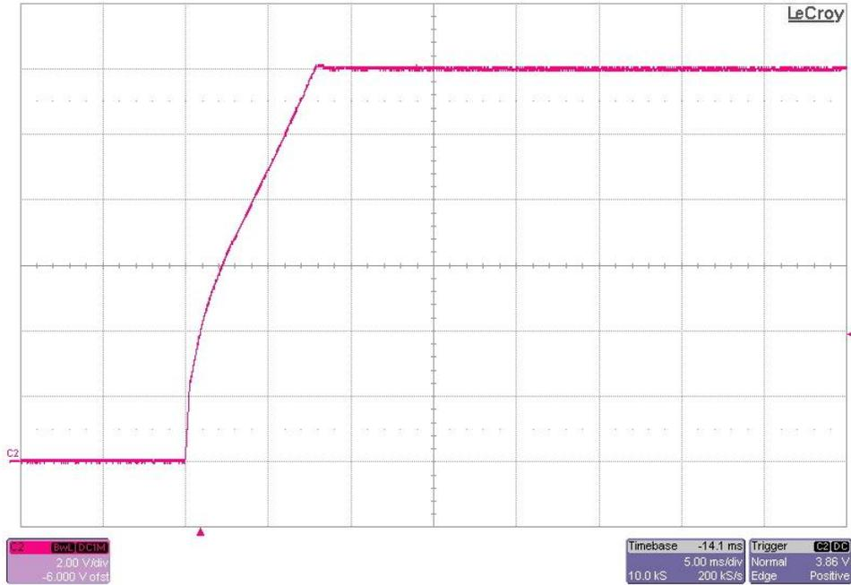
The photo below shows the output voltage startup waveform of a single flyback after the application of 53V in. The 12V output was loaded to 2.5A. (2V/DIV, 5mS/DIV)
