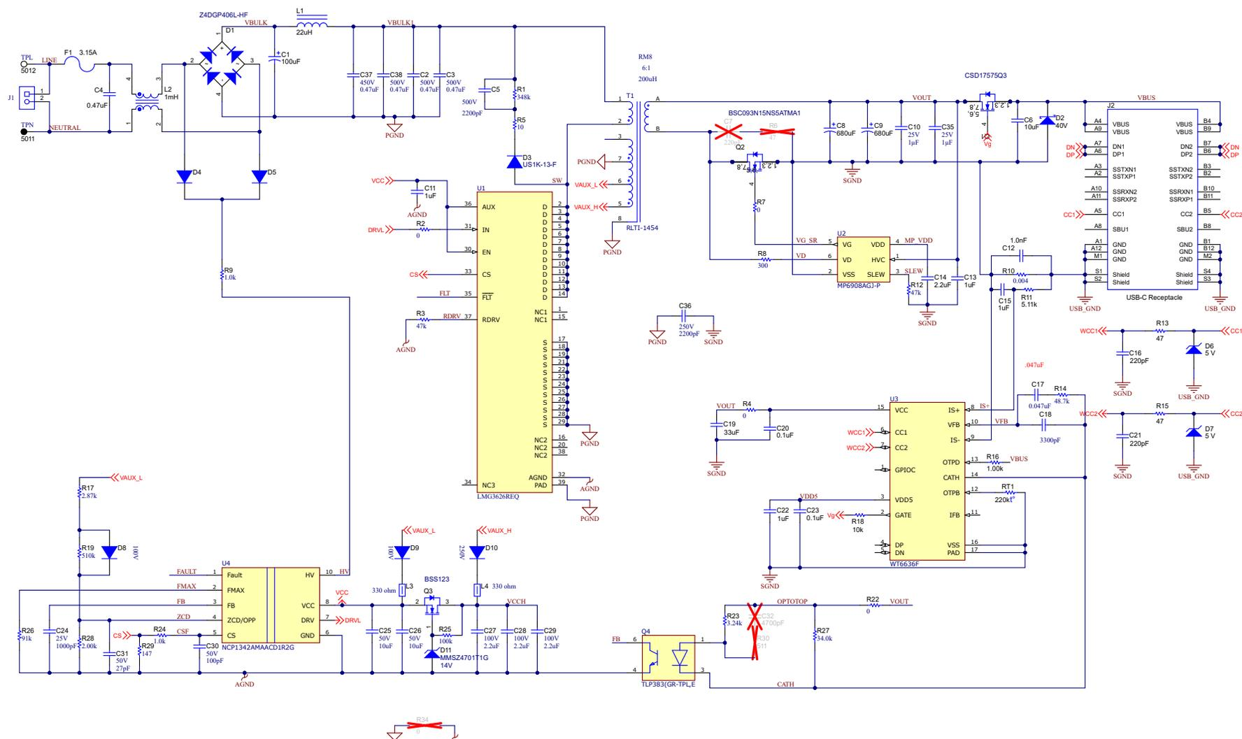
Figure 4-1. LMG3626EVM-074 Schematic Diagram
