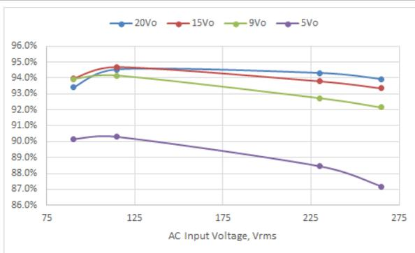
Figure 3-4. Full-load Efficiency vs. Input Voltage
