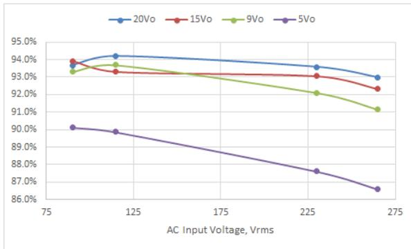
Figure 3-2. 4pt-Average Efficiency vs. Input Voltage
