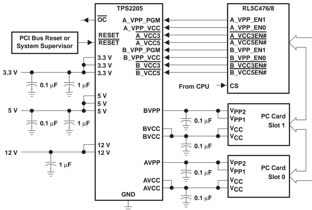
**Figure 5. TPS2205 and Ricoh RB5C478 Application**
