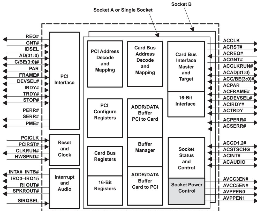
NOTE: A # following a signal name means there is a separate signal for socket A and socket B.
