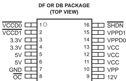
**Figure 3. TPS2211 16-Pin SSOP Package**
