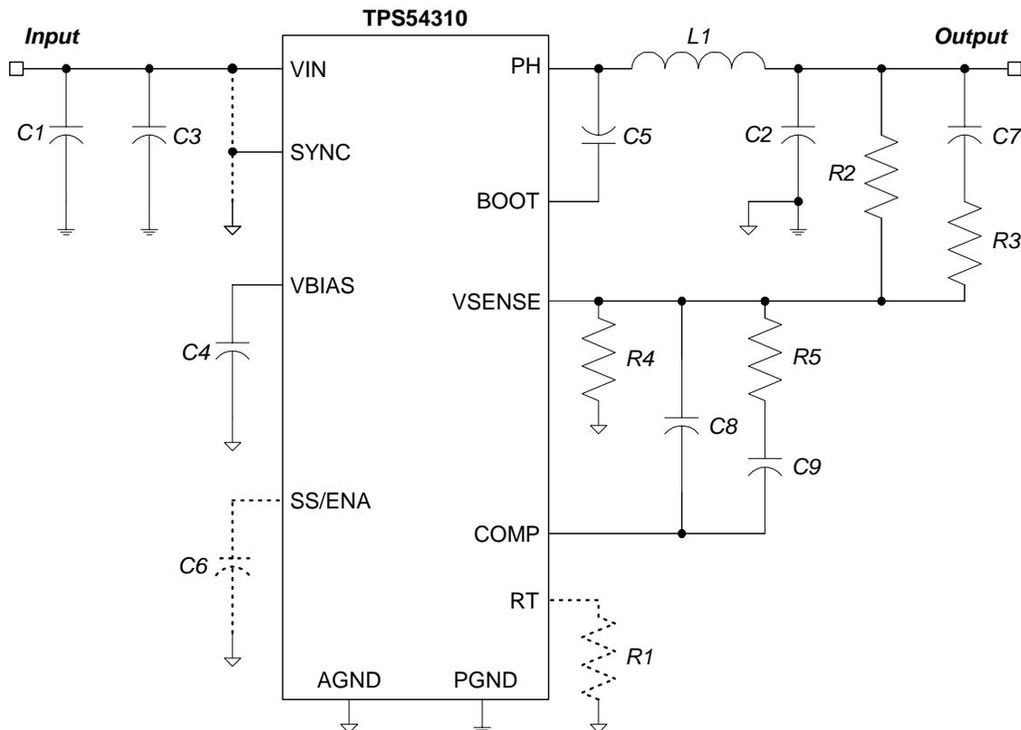
Figure 1. Typical Schematic
