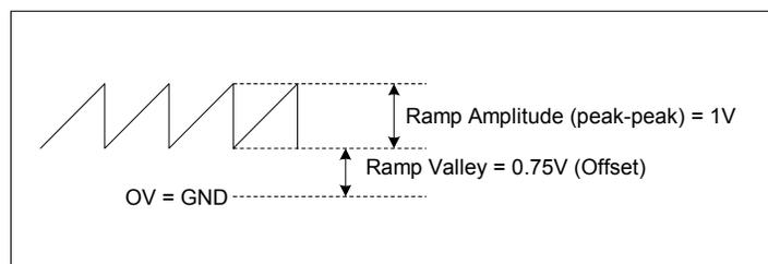
**Figure 3. Ramp Waveform**
