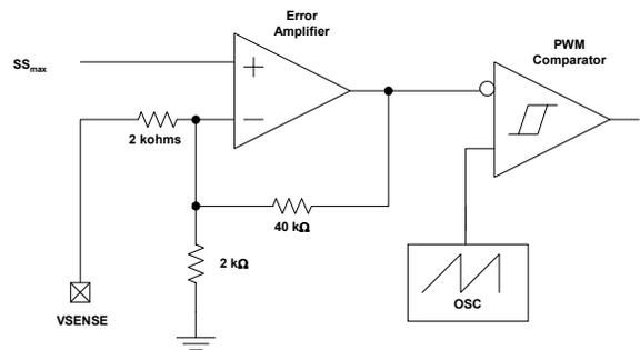
**Figure 2. Feedback Section of the TPS54x14, TPS54x15, and TPS54x16**
