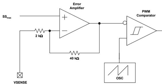
**Figure 1. Feedback Section of the TPS54x11, TPS54x12 and TPS54x13**
