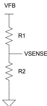
**Figure 4. External Resistor Divider Connection**
