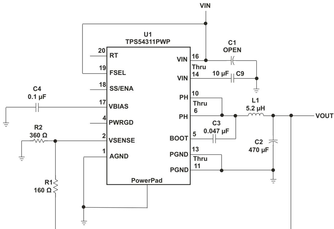
**Figure 8. TPS54311 Schematic Adjusted for VOUT = 1.3 V**
