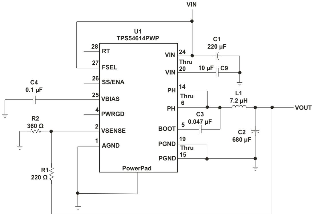
Figure 6. TPS54614 Schematic Adjusted for VOUT = 2.9 V
