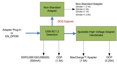
Figure 2-1. DPDM Detection Process
