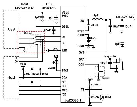
Figure 2-3. Typical Simple Schematic With DPDT Switch
