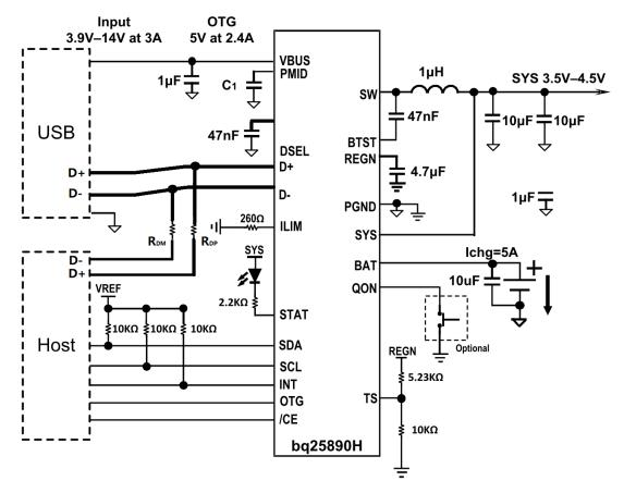
Figure 2-4. Typical Simple Schematic Without DPDT Switch
