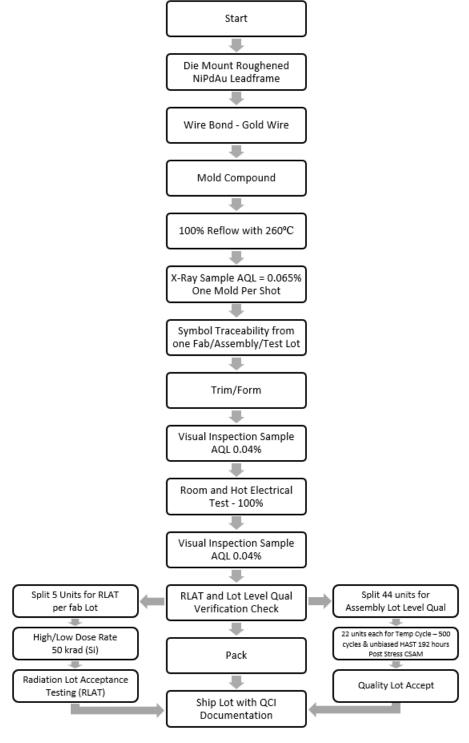
Figure 2-1. TPS7H2201-SEP Space Enhanced Plastic Production Flow Chart
